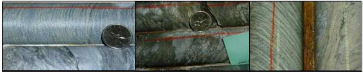
Figure 7.2: Close-up views of typical host rocks (from left to right); finely bedded “Marker” tuff horizon and felsic coarse fragmental volcanoclastic rocks, mineralized felsic volcanoclastic rocks (agglomerate), finely bedded “Marker” tuff horizon
