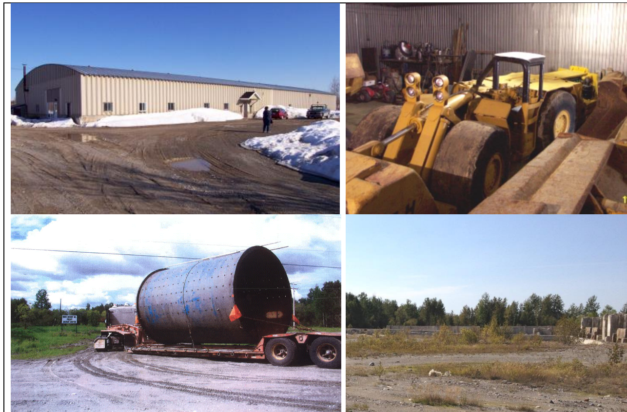
Figure 5.1 : From left to right; External view of the main building, 4 yard Scoop parked in the garage, a ball mill shell being delivered to Abcourt-Barvue, and, in the background, concrete basement of the old mill.
