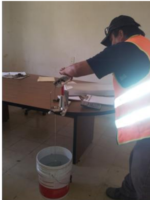
Figure 12.2 Aura Minerals' core shack technician measuring bulk density (December 2014)
