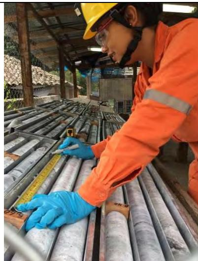
Measurement of the boxes and marking of the meter by meter
