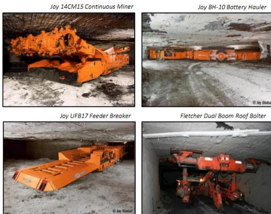
Figure 19: Typical Underground Super-Section Mining Equipment
