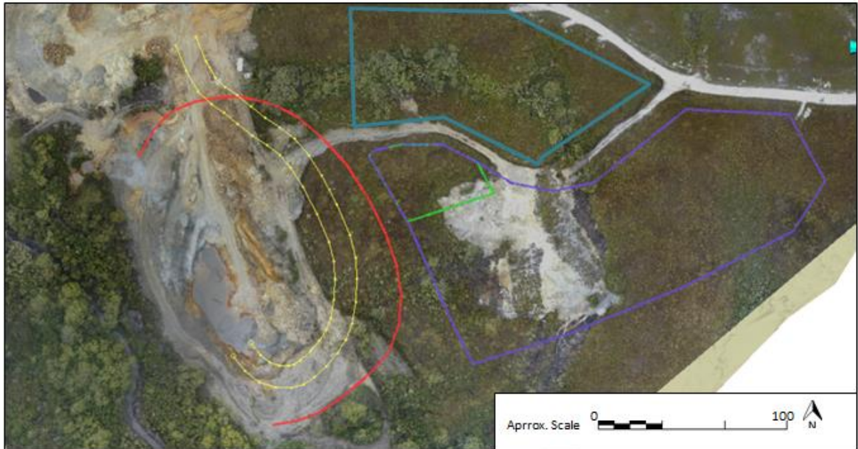
Figure 2.4 - Plan view showing approximate extent of cutback (red), the haul ramp (yellow), WRE (purple), PAF stockpile (green) and ROM stockpile
