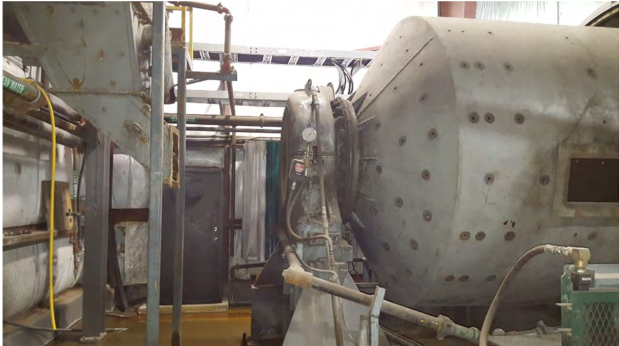
Figure 17.4 Primary Ball Mill
