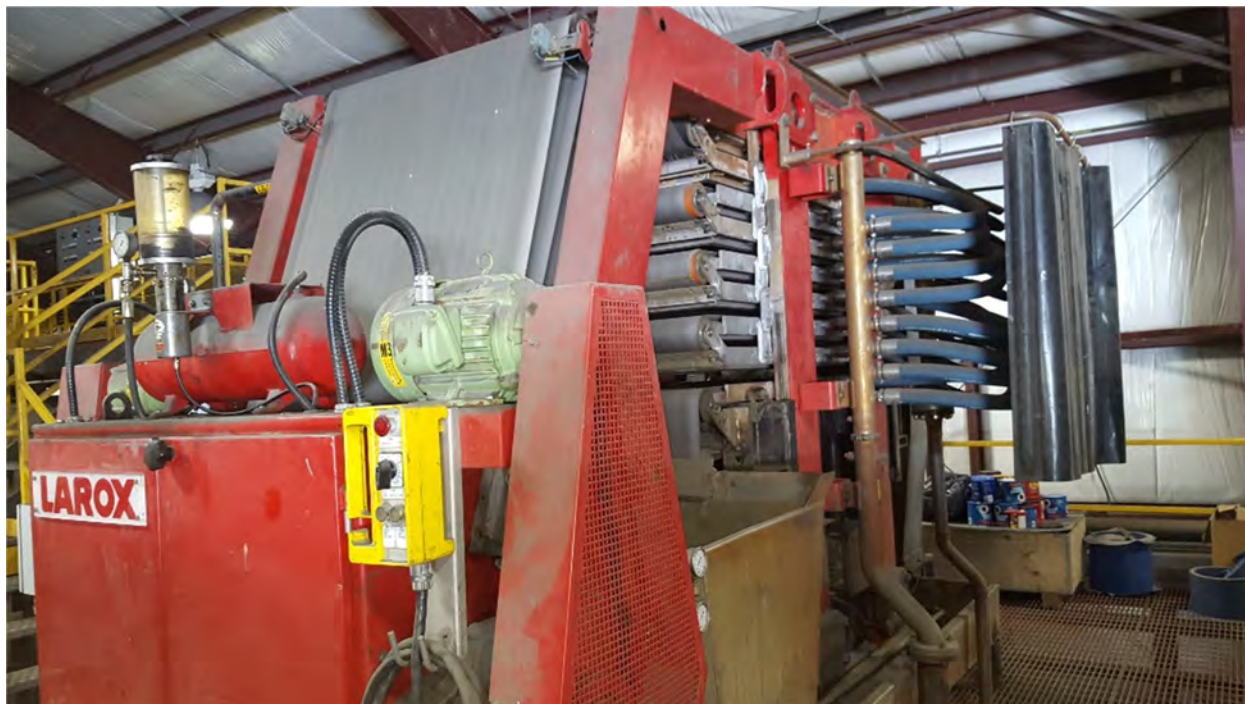
Figure 17.6 Larox Pressure Filter
