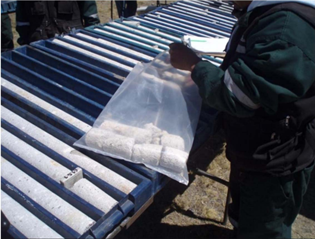
Figure 11-1: Whole Core Samples are Bagged on Site
