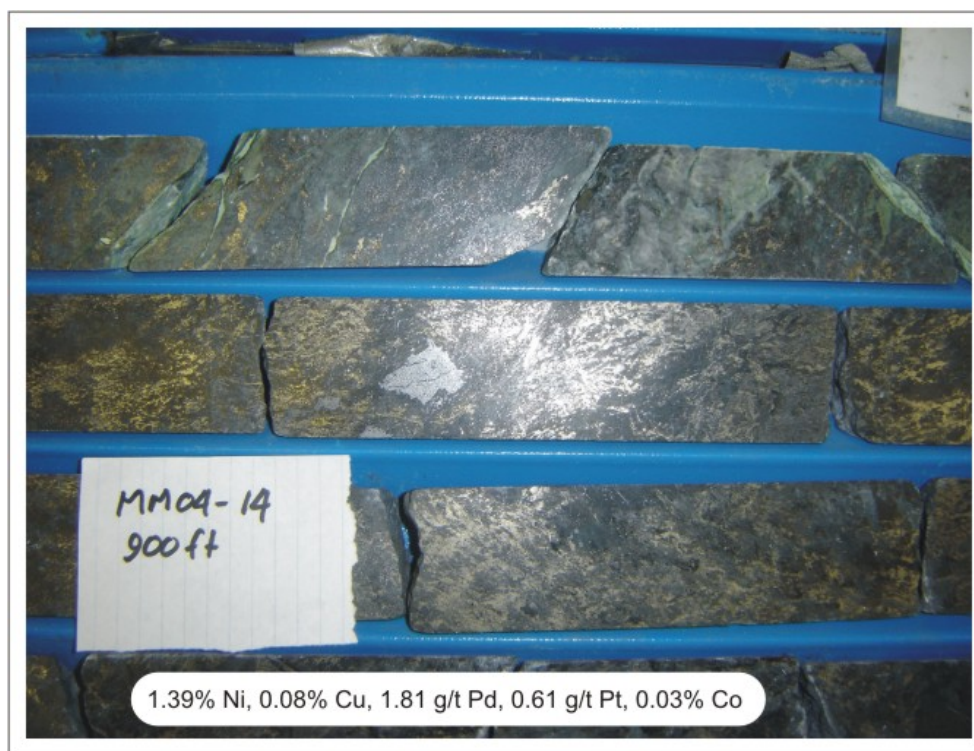
FIGURE 14-9 VIEW OF HIGH GRADE NICKEL MINERALIZATION (SULPHIDE ZONE), DRILL HOLE MM04-14, MAKWA PROPERTY
