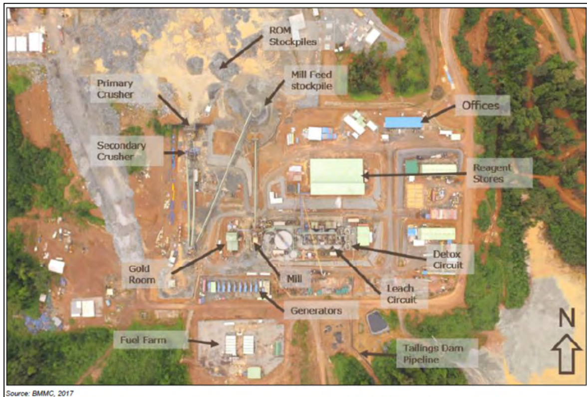
Figure 17-1: New Liberty existing plant layout
