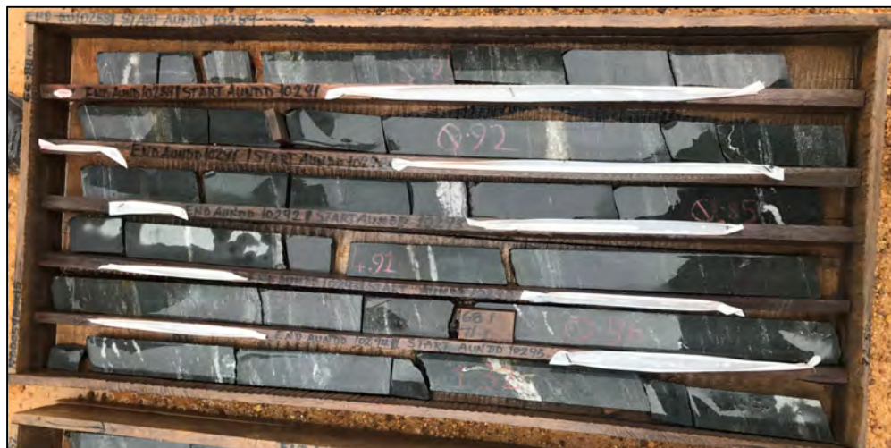
Figure 12-3: NDD059 – drill core shown within 70–73 m, with an average weighted grade of 2.26 g/t Au
