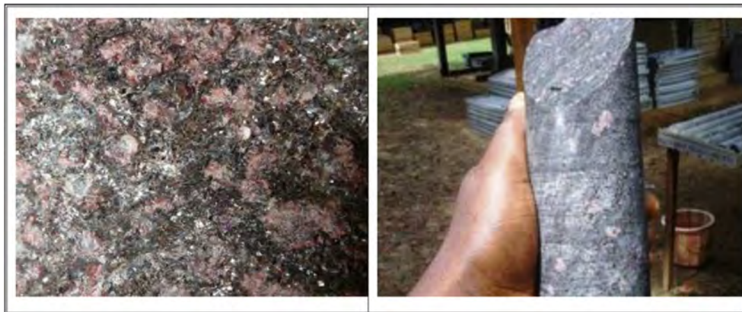
Figure 7-5: Almandine garnet porphyroblasts in HWC Source: BMMC, 2017
