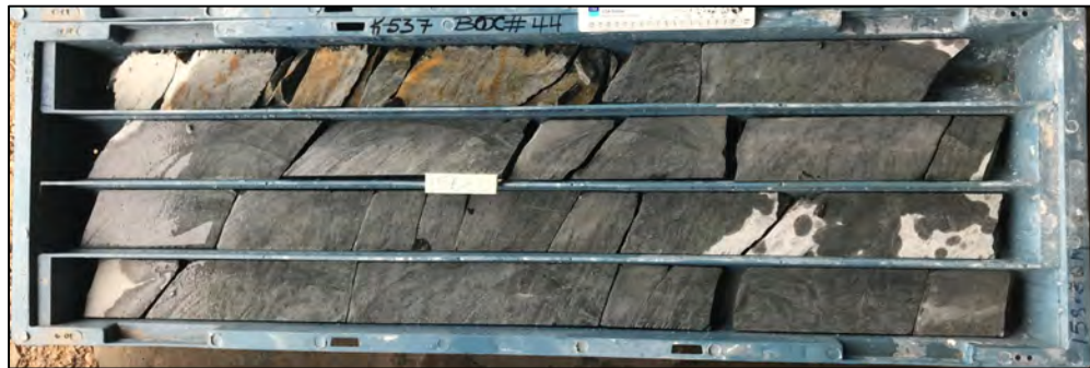
Figure 12-2: K537 – drill core shown within 155–159 m, with an average weighted grade of 2.13 g/t Au
