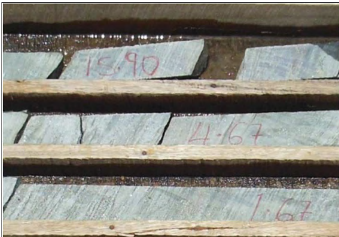
Figure 7-8: Sheared ultramafic schists (mineralised zone) Source: AMC, 2014
