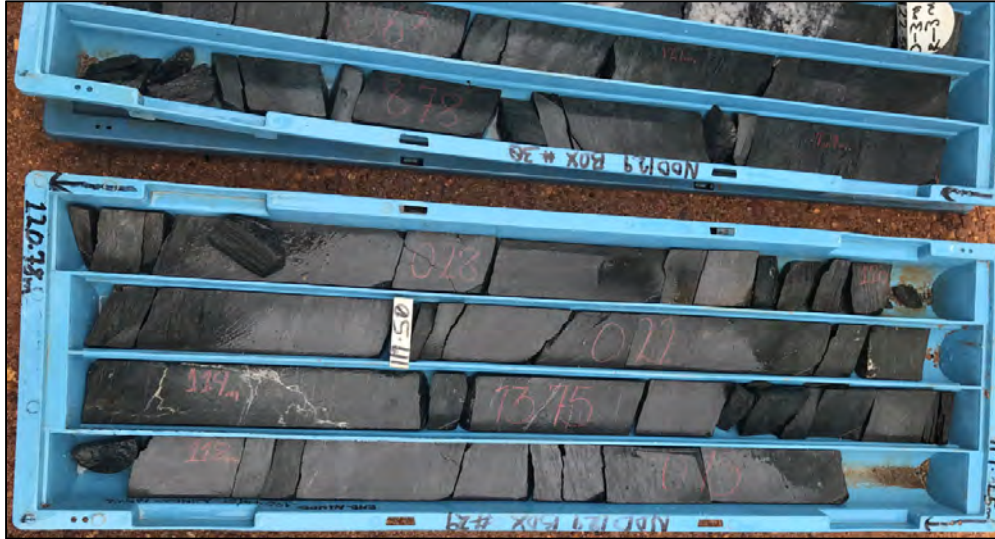
Figure 12-4: NDD129 – drill core shown within 117–122 m, with an average weighted grade of 4.64 g/t Note: Host rock is phlogopite-tremolite-chlorite schist. Source: CSA Global, 2018
