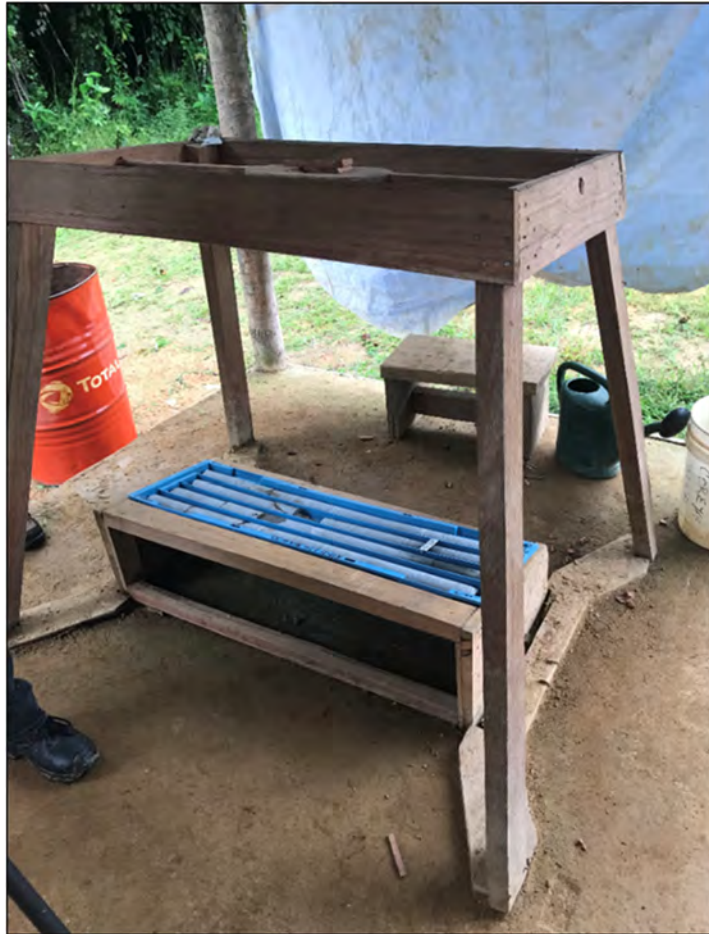
Figure 10-3: Ndablama drill core photograph structure Source: CSA Global, 2018
