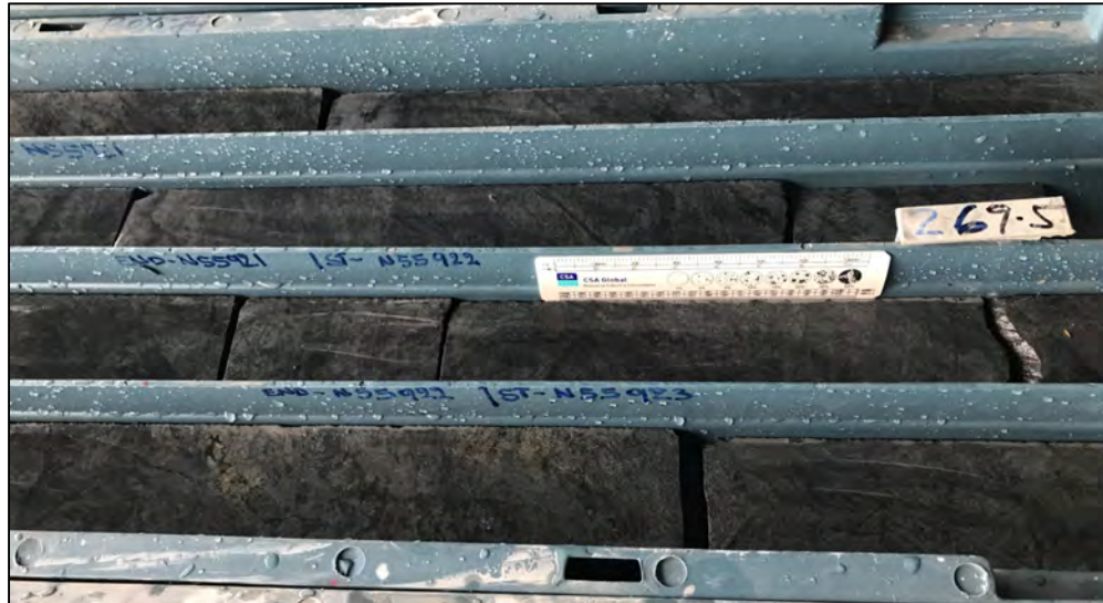
Figure 12-1: K501 – drill core shown with locations of samples N55921, N55922 and N55923 (269–272 m, weighted average grade 11.99 g/t Au)
