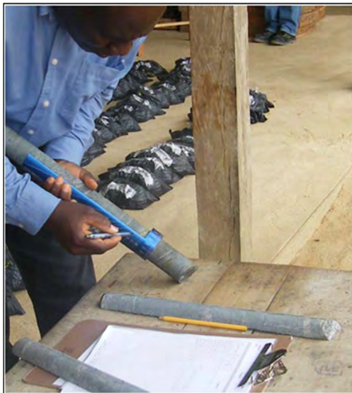
Figure 10-4: Structural core measurements Source: AMC, 2014
