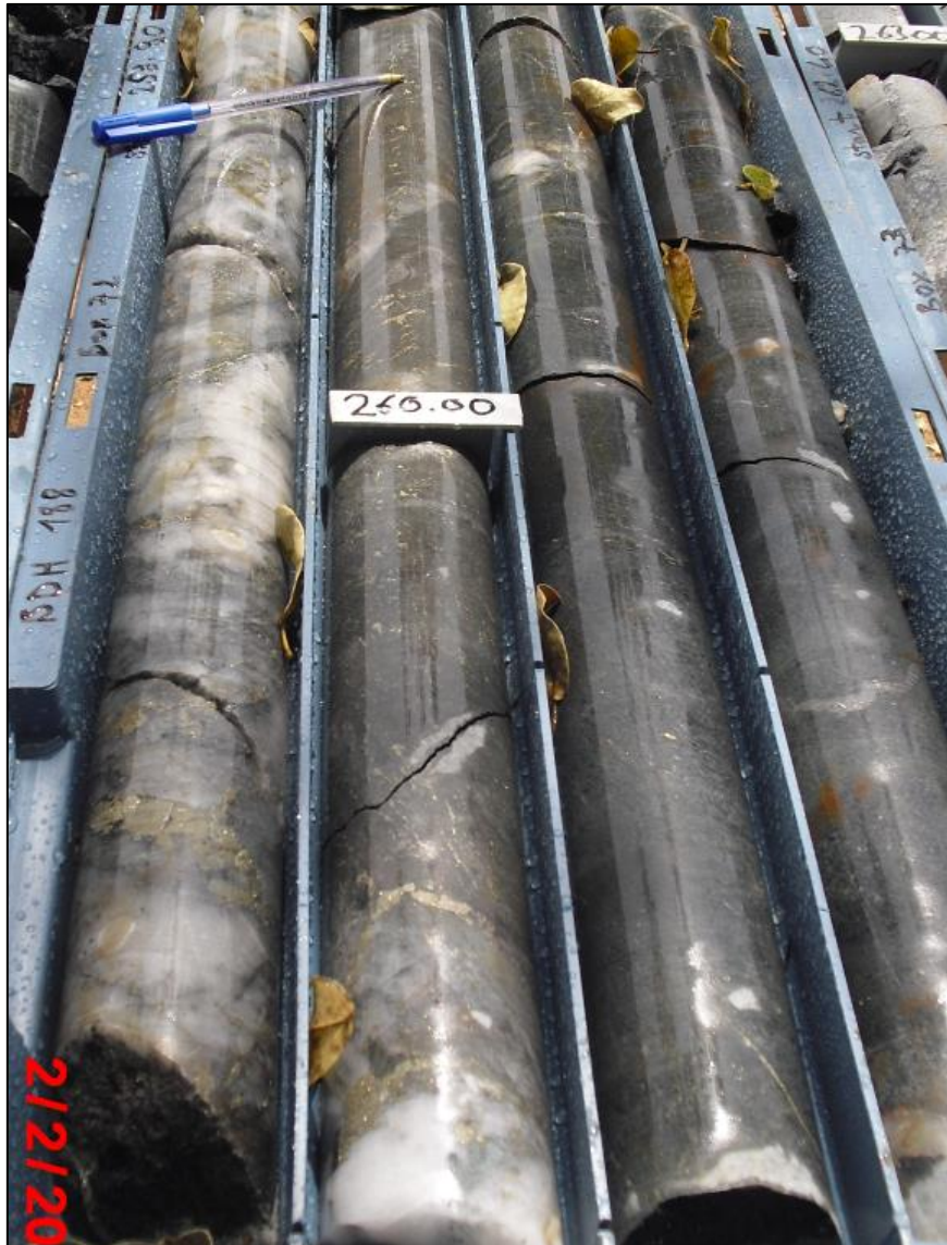
Figure 7-11: Drill core from hole BDH188, Netiana lodes, Balogo property, 258.5 m to 262.4 m, showing thick quartz vein and possible high-grade mineralisation
