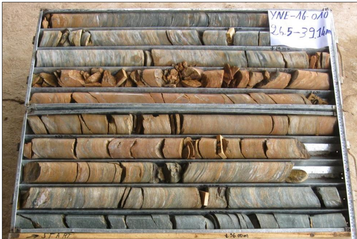
Figure 7-9: Mineralised core at A2N East, core shown averaging 3.7 g/t, highest grade is in the first 3 m of the lower core tray including 21 g/t between 32.15 m and 32.5 m
