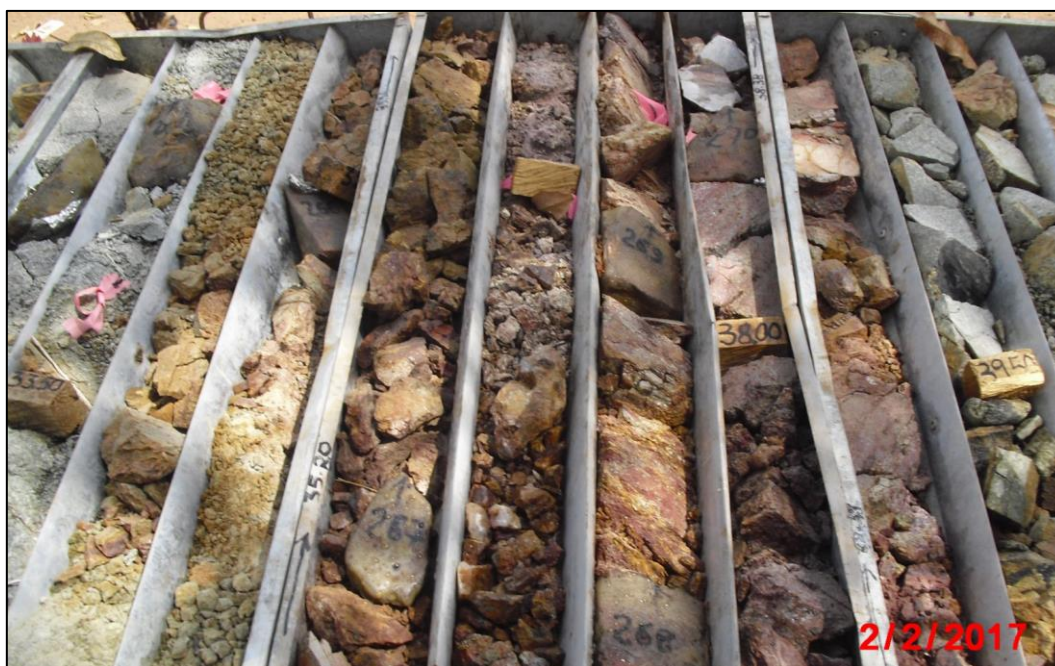
Figure 14-8: Drillhole BDH046 (Netiana lode, Balogo property) showing weathering profile and billets chosen for BD measurement
