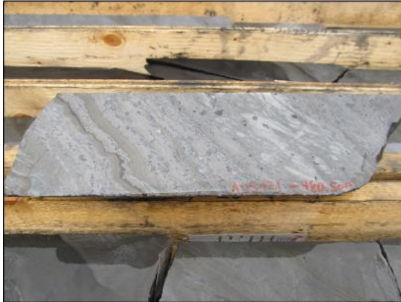
Figure 10-15: Mottled Textured High-Grade Mineralization in A-15-121 @ ~480.50 m
