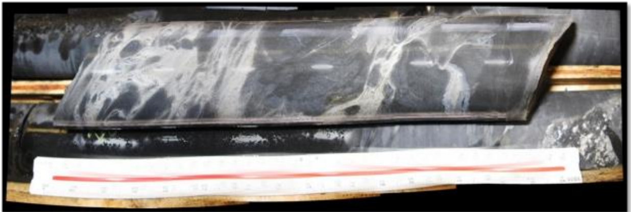
Figure 7-17: Sphalerite-Rich Sulphide Breccias in Road River Rocks in A-08-63 @ 479 m
