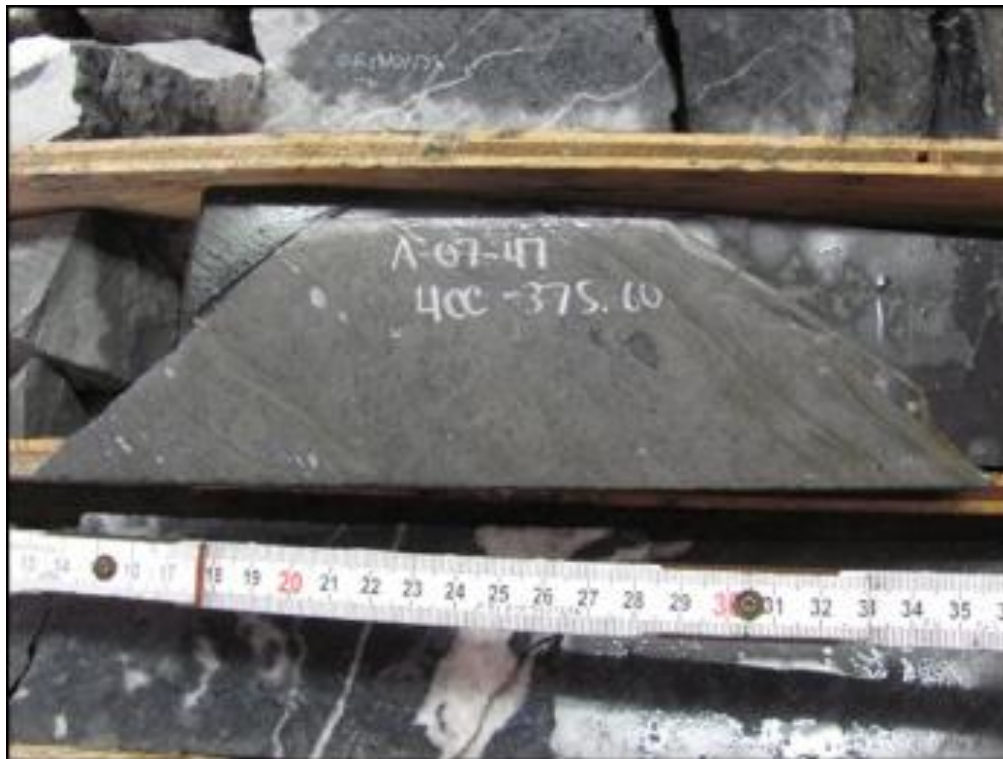
Figure 7-11: Mottled Textured High-Grade Cardiac Creek Zone Mineralization in A-07-47 @ 375.60 m
