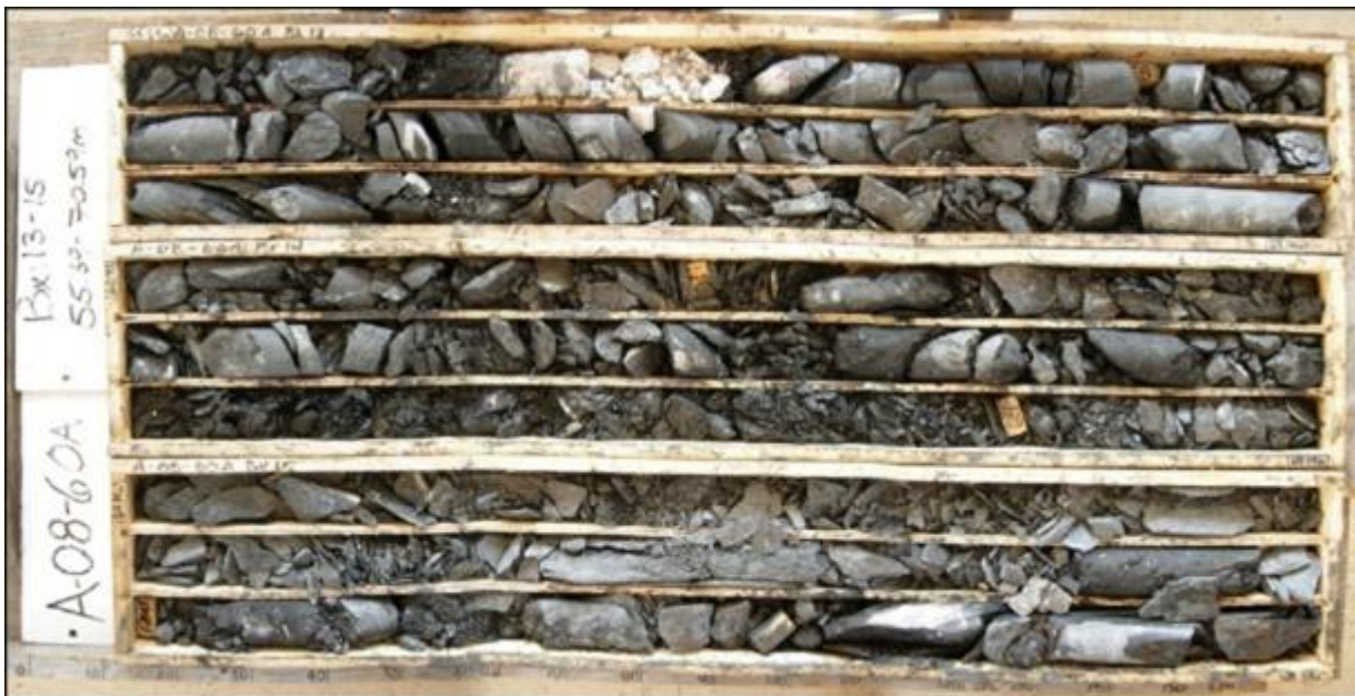
Figure 10-22: Bad Ground Associated with Brittle Faulting (A-08-60A)
