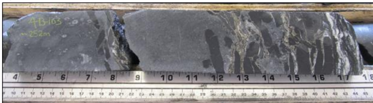
Figure 10-12: “Nick” Style Mineralization in Hole A-13-103 @ 252.37m
