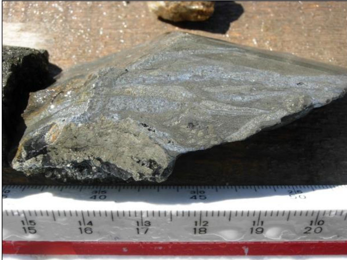
Figure 10-6: A 5 cm Piece of the 0.8 m Interval of Massive Sulphide in A-96-24
