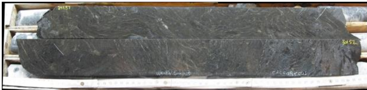
Figure 10-11: “Nick” Style Mineralization Intersected in A-10-72 @ 299.57 m
