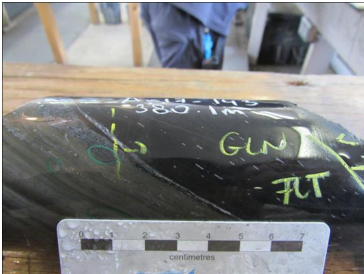
Figure 10-27: Remobilized Galena within Gunsteel Formation Shale in A-17-143 @ 380.10 m
