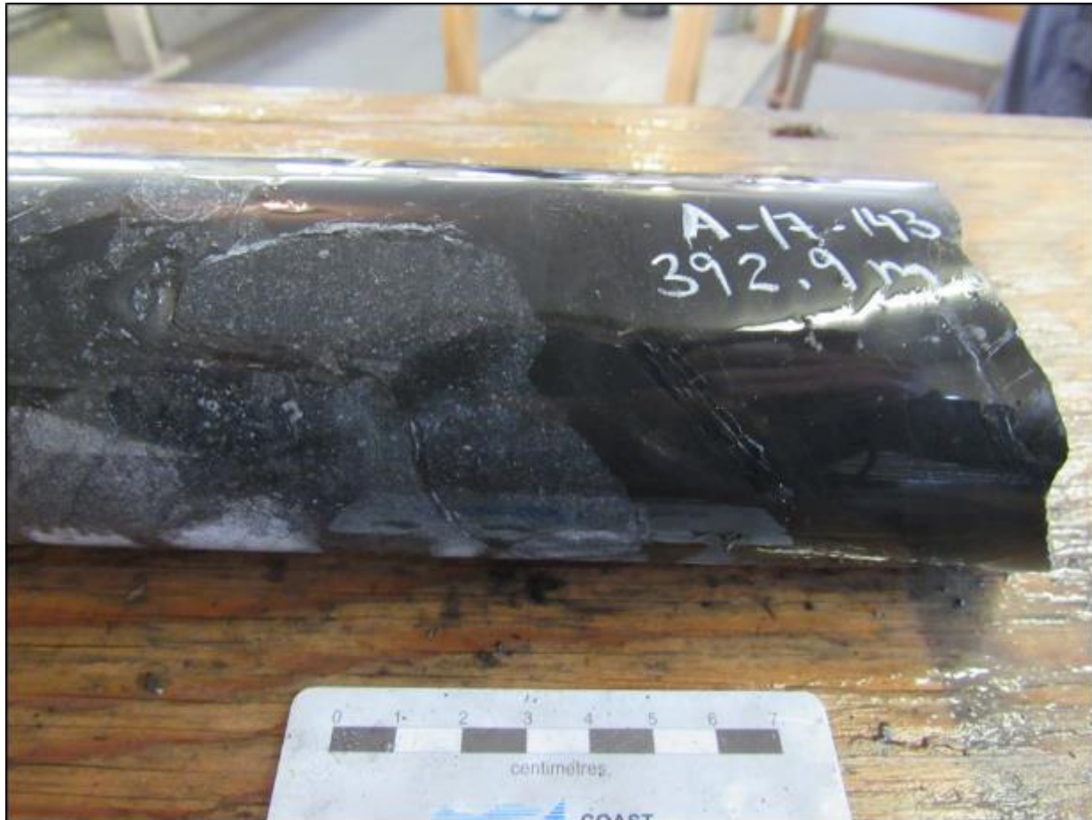
Figure 10-26: “Nick”-style Mineralization in a-17-143 @ 392.84 m
