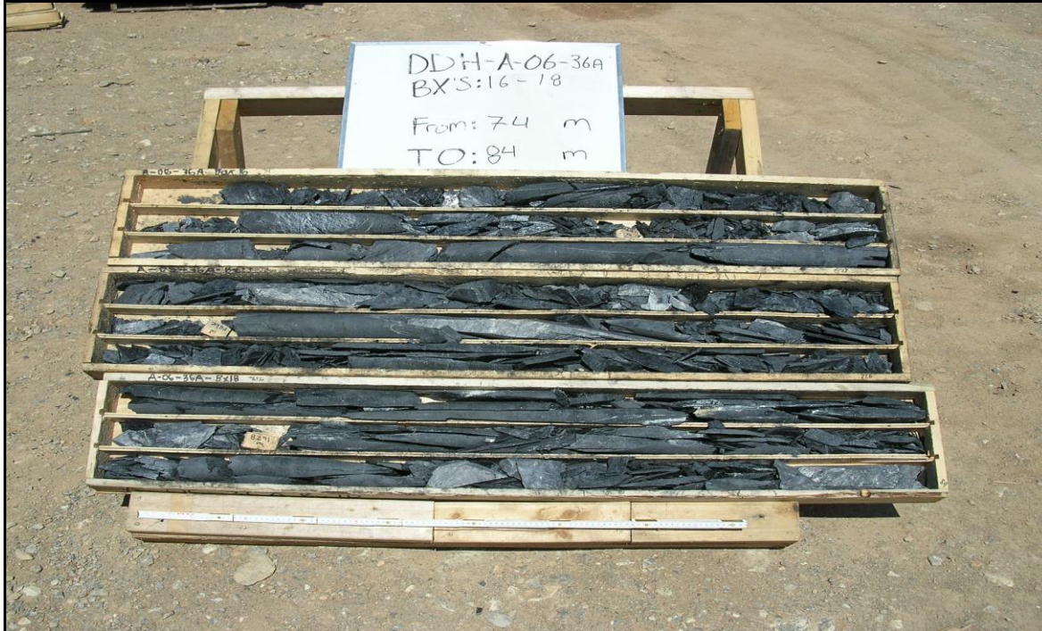
Figure 10-21: Fissile Character of the Gunsteel Formation Shales (Hole A-06-36A)
