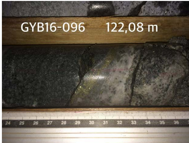
Photo 3: Drillhole GYB16-096, cte-py-qtz veinlet @5.25 g/t Au, 11.3 g/t Ag, hosted in a tonalite with weak propylitic alteration.
