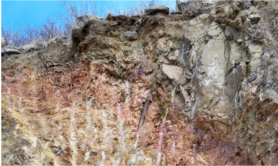
Figure 12.14: Uranerz BX Sized Drill Casing Exposed in Road-Cut
