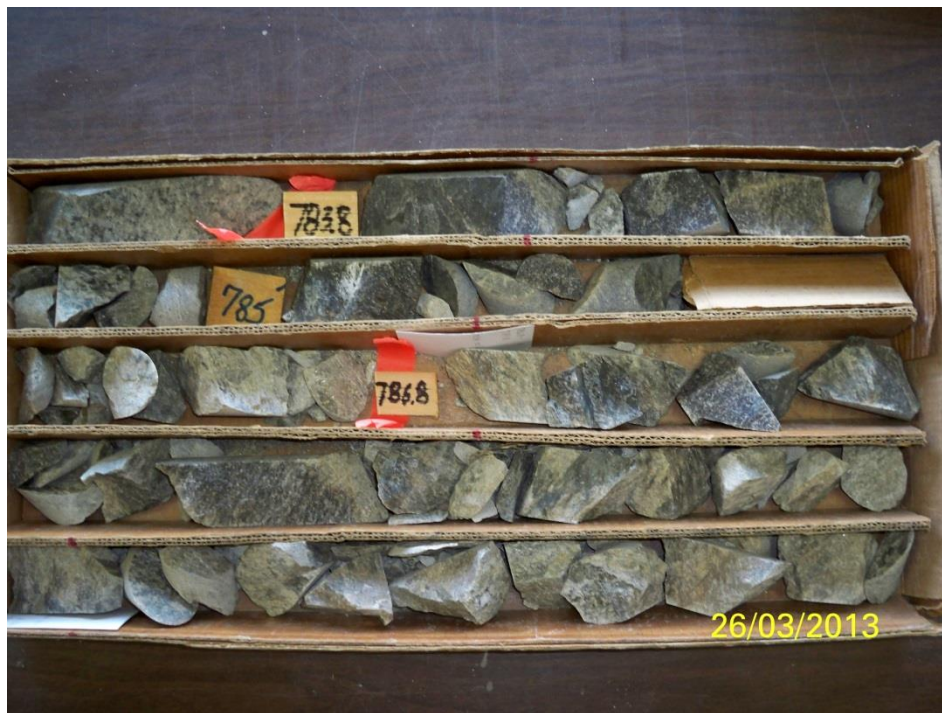
Figure 12.6: Felsic Biotite Gneiss in US Borax Hole GC44 (check sample 783.8–786.8 ft)
