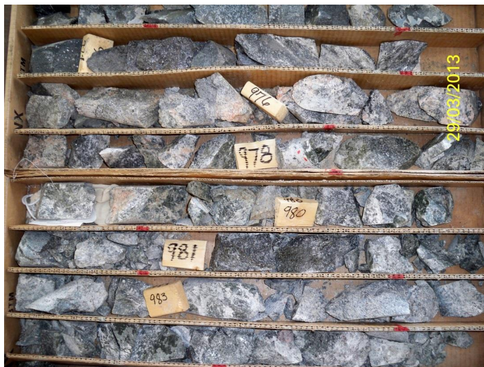
Figure 12.7: Felsic Biotite Gneiss in Uranerz Hole DA9007 (check sample 978.0–981.0 ft)
