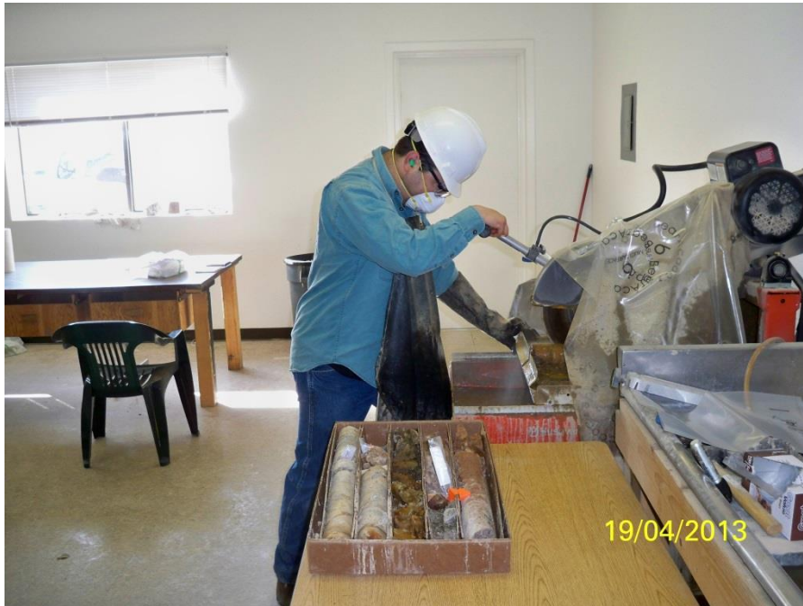
Figure 12.16: Zephyr Geo-Technician Sawing HQ-Sized Core
