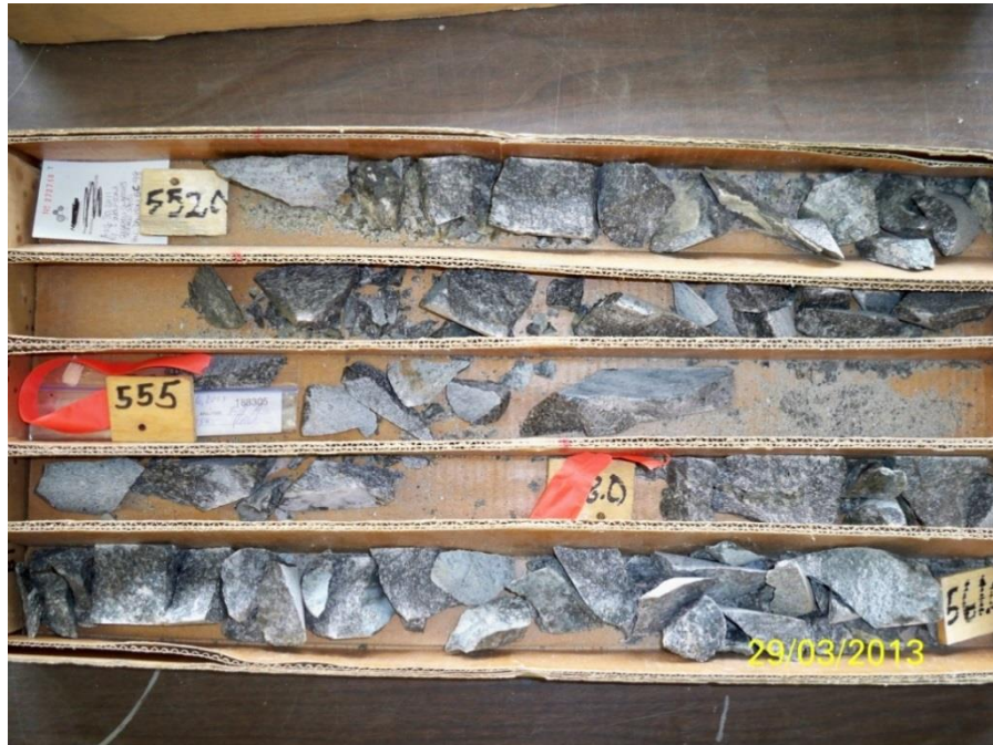
Figure 12.8: Felsic Gneiss in Jascan Hole GC98 (check sample 552.0–555.0 ft)
