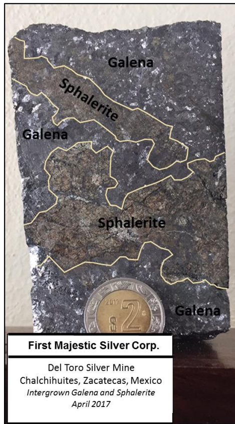
Figure 7-8: Ore from Perseverancia Showing Intergrown Galena and Sphalerite
