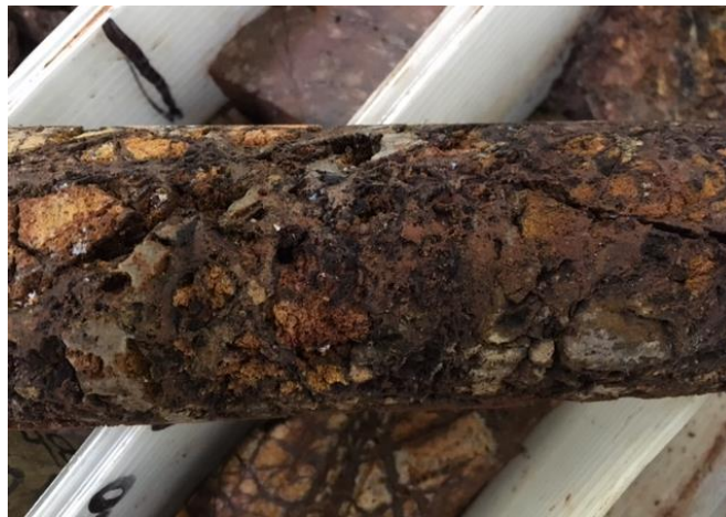
Figure 16-2: Highly Leached and Oxidized Skarn
