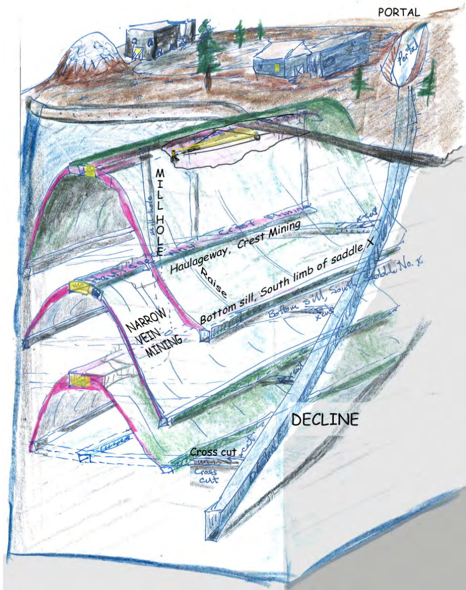
Figure 16-2: An illustration of the proposed mining method.
