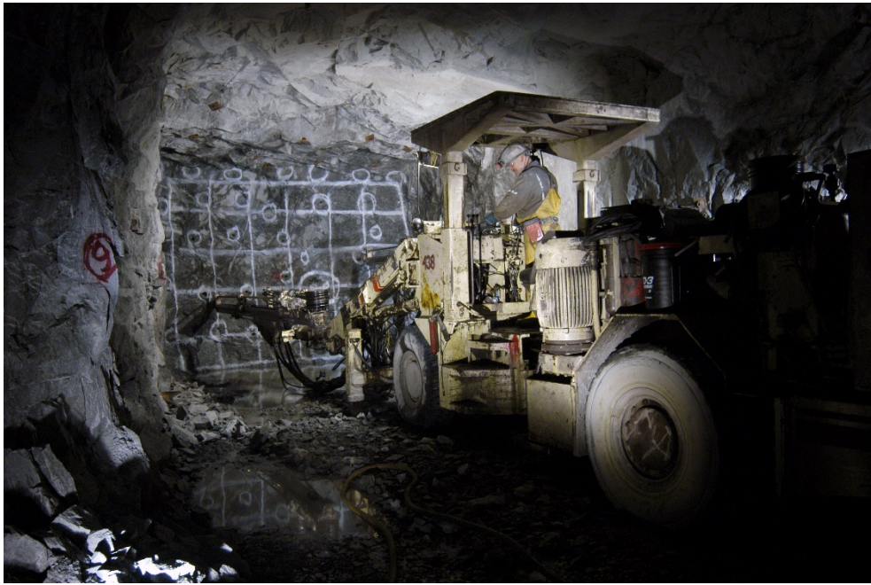
Eagle River Mine – Electric-hydraulic Jumbo Drill Advancing 750 metre level drift to the 300 zone
