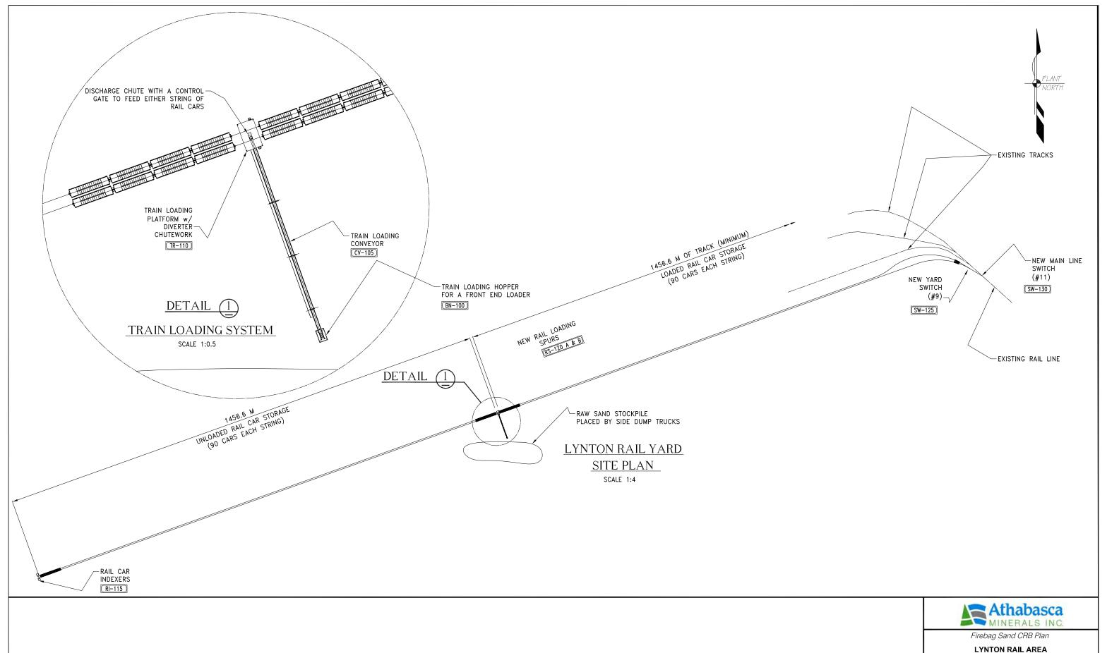
LYNTON RAIL AREA SITE PLAN AND LOADOUT DETAIL
