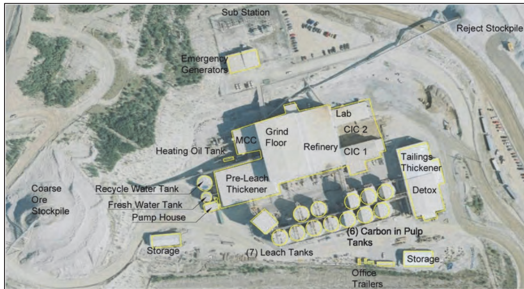
Figure 17-2: Fort Knox Mill Complex Site Plan.
