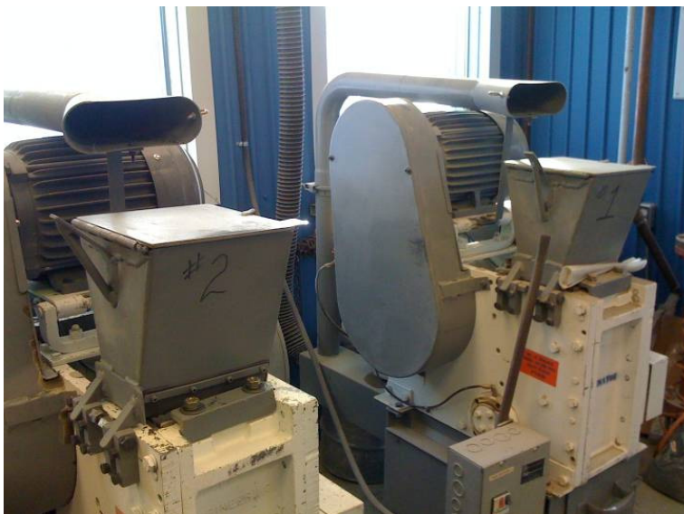
Figure 10-3: Sample dryer (top left), drying pan (top right) and jaw crushers (bottom).
