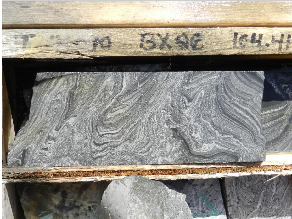
Figure 19: Chaotic folds related to soft-sediment deformation in gray facies mineralization from Tom West Note: NQ diameter drill core from TYK-010 drilled in 2011 (depth 104.7 m).
