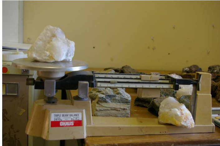
Figure 11-4 Dry sample weighing using an OHAUS triple beam balance
