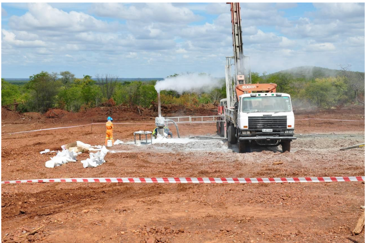
Figure 11-2 Exploration RC drilling adjacent to Tholo open pit. Photo looking south.
