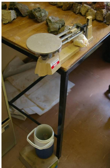
Figure 11-5 Wet sample weighing, with rock suspended in water beneath the triple beam balance
