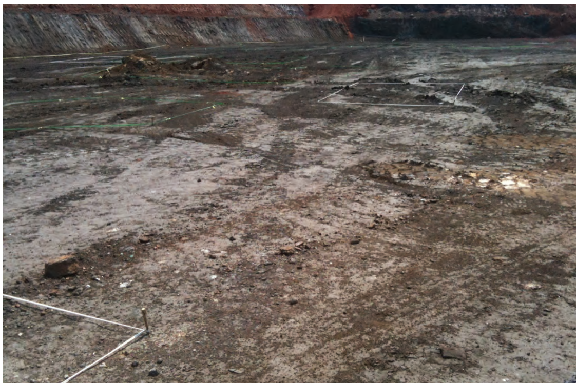
Figure 36: Grade control demarcation
