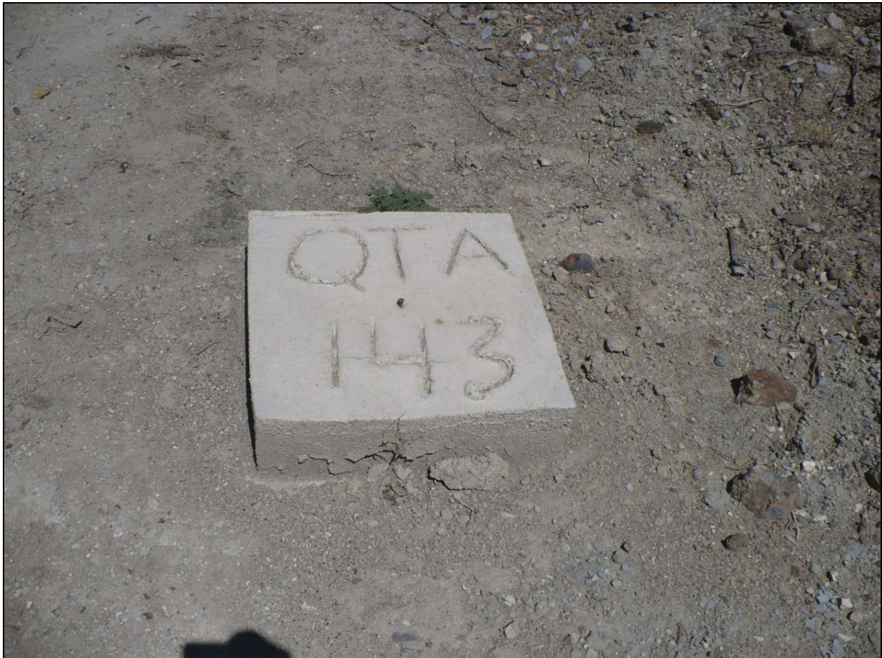
Figure 10-1: Typical Drill Hole Cap and Marker
