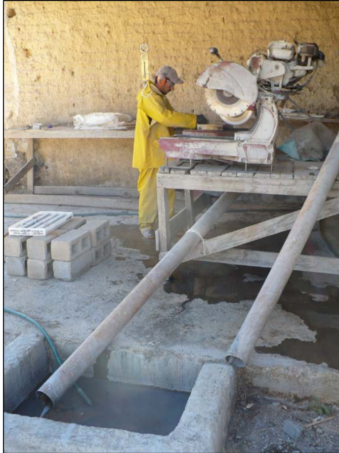
Figure 11-1: Core Cutting and sample prep area at core logging / core storage facility
