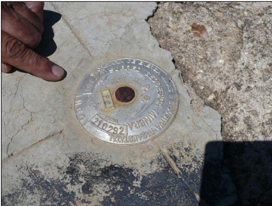
Figure 12-5: Federal survey claim marker with datum peg showing date, datum and federal identification number
