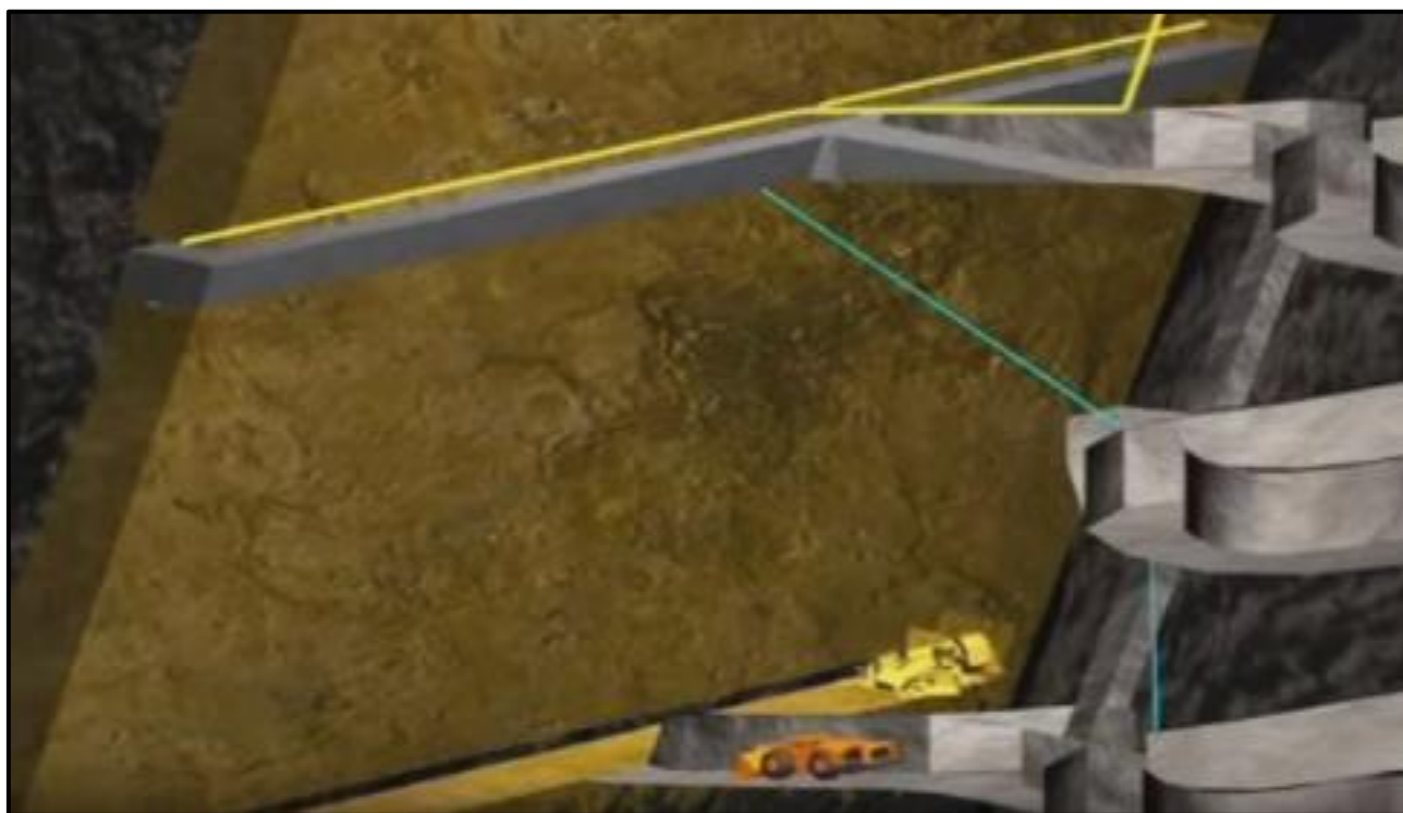
Figure 16.7 – Cut and Fill Mining Method, showing the main decline, raises, vein and services.
