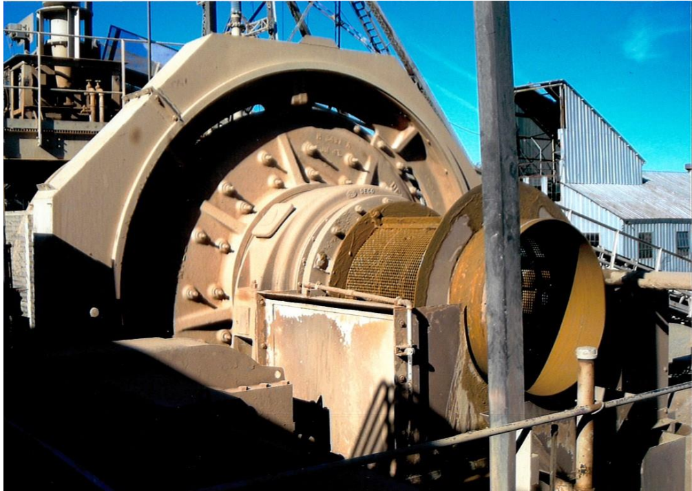
7-ft x 10-ft, 300 HP, Denver ball mill.
