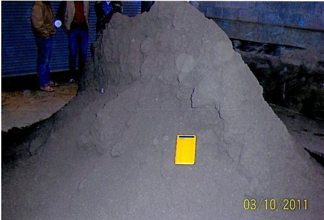
Ten tons of flotation concentrate. The grade is approximately 9 oz Au per ton and 500 oz Ag per ton.
