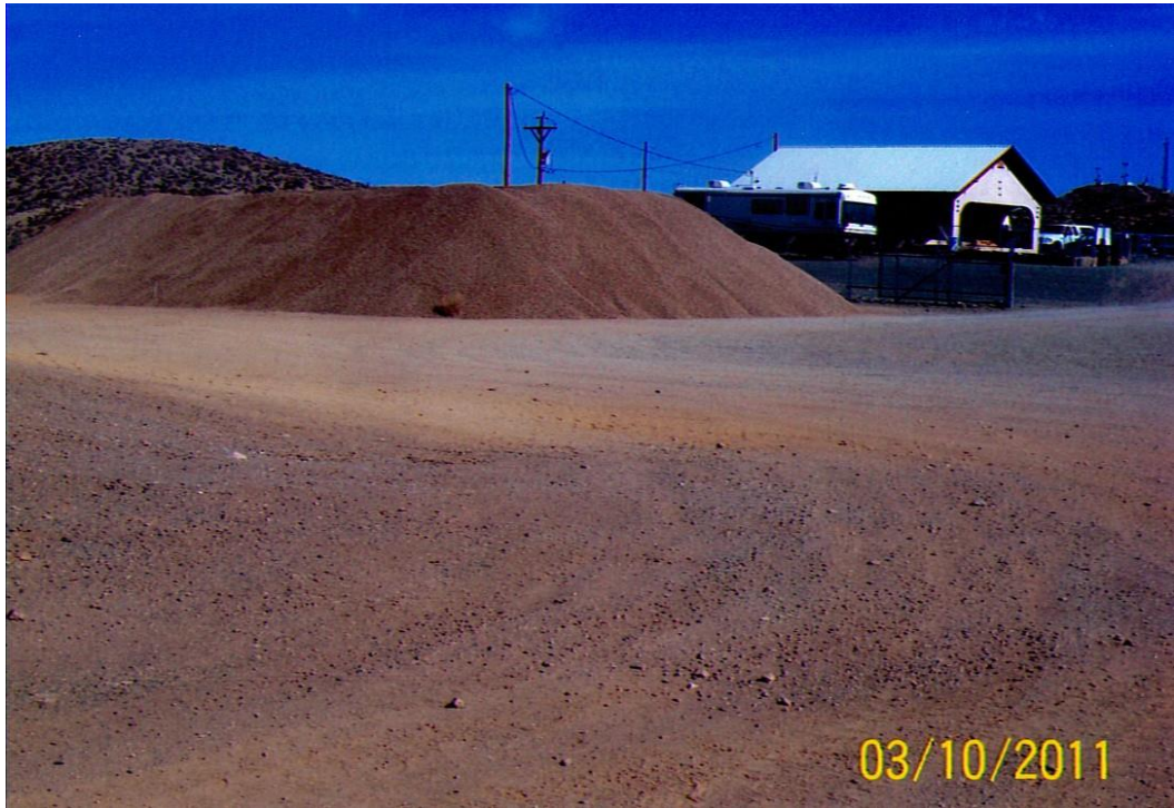
A 1000-ton lot of sized silica flux ready for shipment. The grade is approximately 0.10 oz Au per ton and 10 oz Ag per ton.
