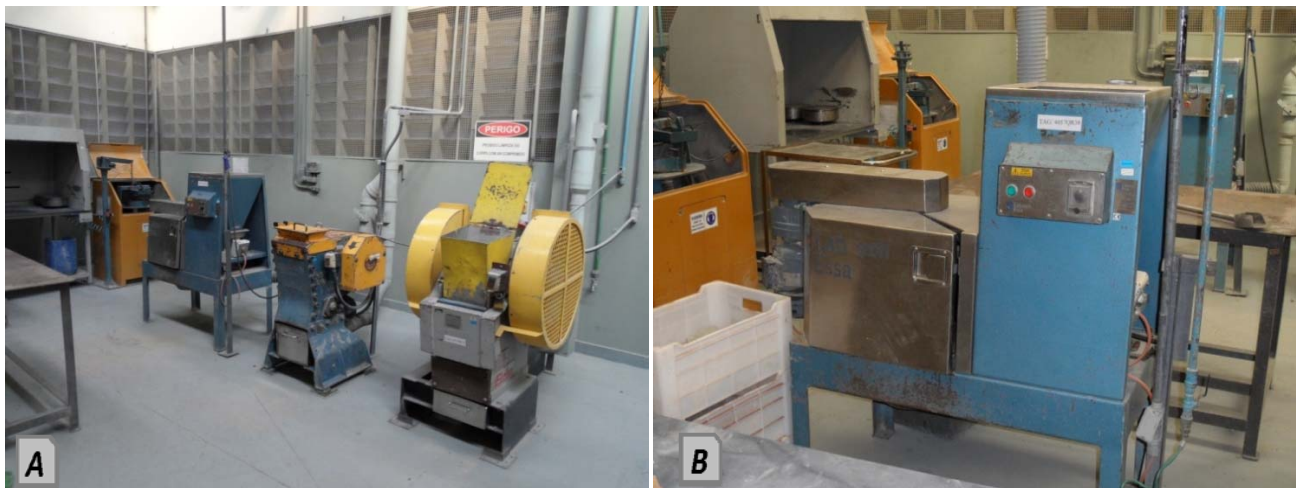
Figure 8-16: A) General view of laboratory mechanical sample preparation equipment. B) Rotary splitter
