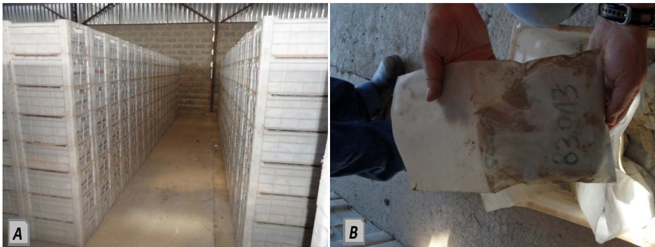
Figure 8-14: A) General view of pulp and coarse reject storage area. B) Plastic bag containing pulp rejects
