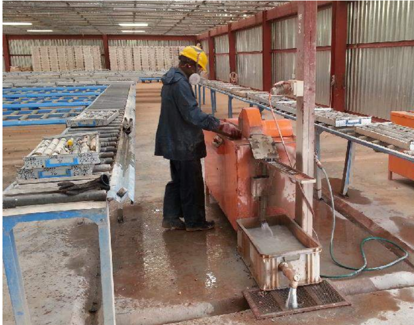
Figure 11-2 Sawing core samples (November 2013 Site Visit)
