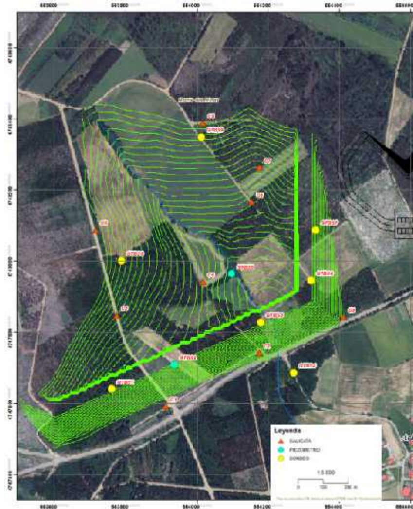
Figure 18.2 - Geotechnical investigation campaign. Borehole and Test Pit Locations. (Terratec 2016)
