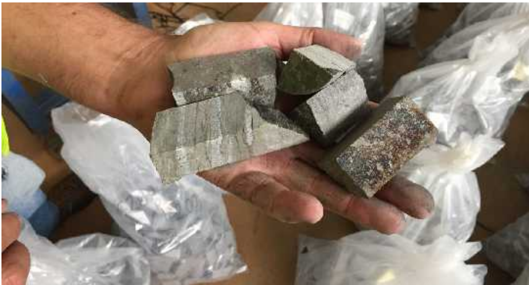
Figure 13.1 - Typical Drill Core Photo (Photo taken by T. van Bockxmeer, Minovo 2016)
