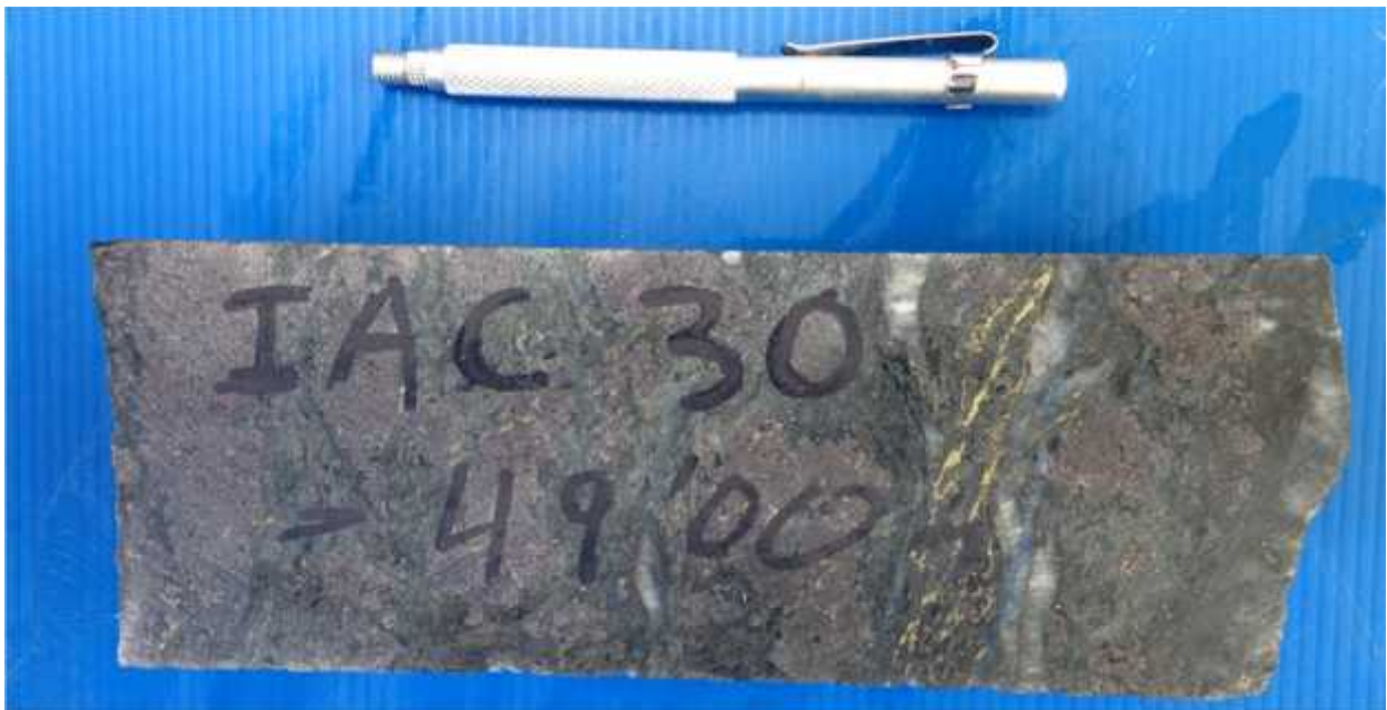
Figure 7.8 – Garnet amphibolite in Arca, hole IAC30 (Atalaya 2017)
