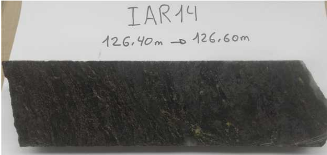
Figure 7.6 - Mineralized specimens of Arinteiro garnet amphibolite, hole IAR14 (Atalaya 2017)
