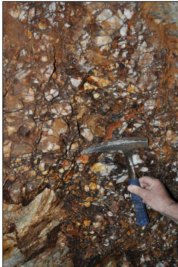
Figure 7-4. Brecciated Quartz Veins Exposed In Adit
