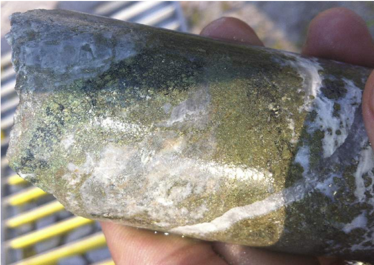
Plate 3: BK029, 90m – Covellite disease of massive pyrite.
