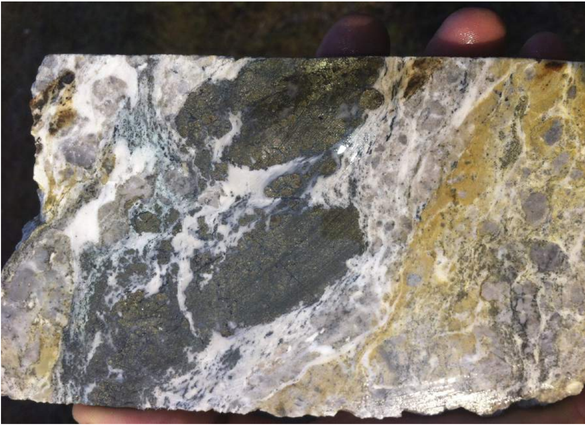
Plate 4: BK032, 29m – Fluid saturated shear/tectonic breccia. Milled Si fragments and exfoliating and sheared py. Cu staining observed with covellite diseased fine or milled py.
