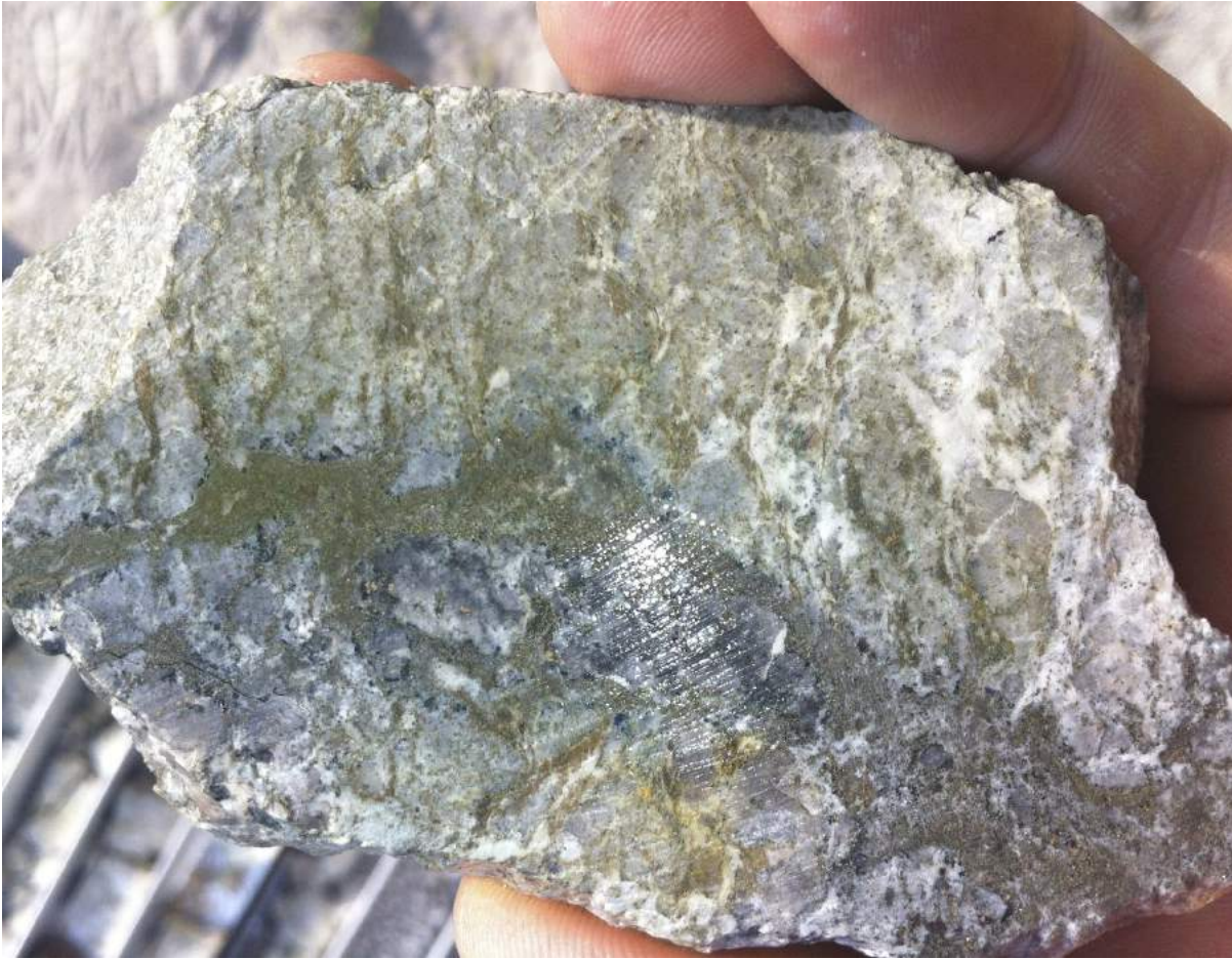
Plate 1: BK029, 15m – Covellite disease of fine pyrite along vein margins. Strongly sheared/milled and foliated silica-clay altered rock
