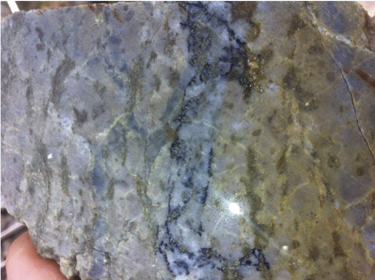
Plate 2: BK029, 39m – Covellite disease of fine pyrite along vein margins. A later blebby pyrite alteration event overprints covellite, evidence that Cu mineralisation replacing pyrite is from a hypogene event. Strongly sheared and foliated rock.
