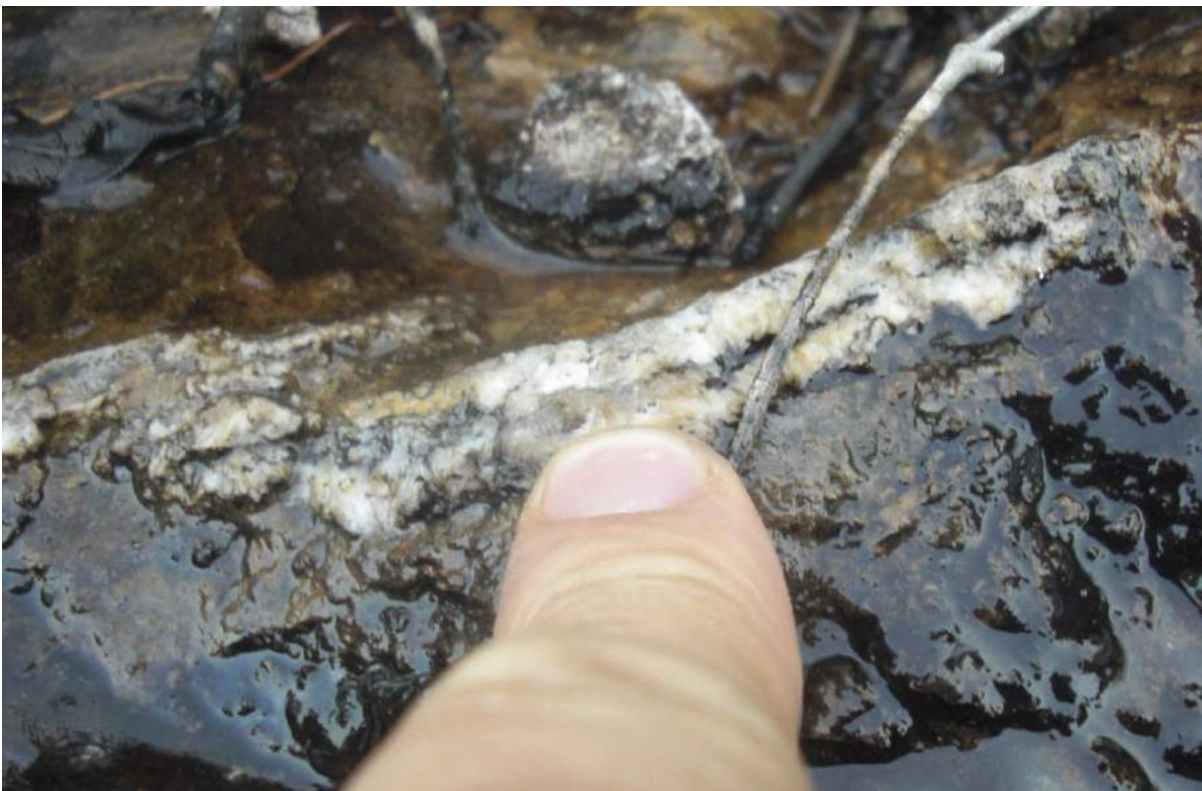
Photo 4: Quartz vein with cast following leaching of pyrite. Association and texture similar to veins observed in core.
