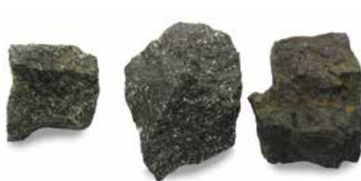
Figure 3a: Samples of massive (right), heavily disseminated (middle) and lightly disseminated (left) ore, typical of the lower vanadium-bearing magnetite at the Brits Vanadium Project
