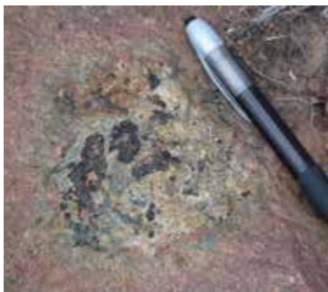
Figure 6a: Large cassiterite (SnO 2 ) crystals in granite at the Groenfontein Tin Mine (Mokopane Tin Project)
