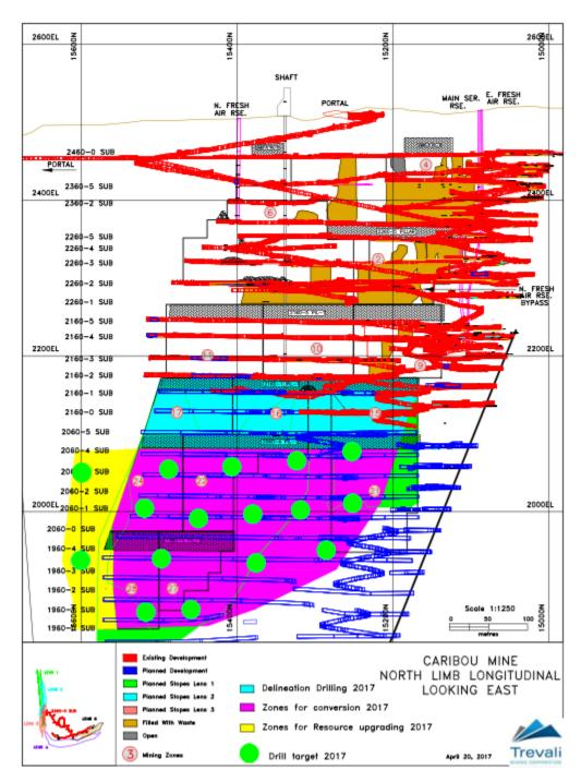
Figure 2: Caribou Mine – North Limb 2017 underground drill program plan.
