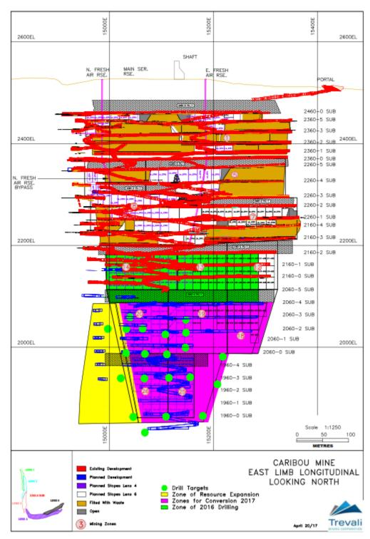
Figure 3: Caribou Mine – East Limb 2017 underground drill program plan.
