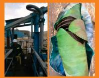
The flexible hose, installed under tension at the bend, ruptured to acid degradation. Acid leaks could not be detected since the sock covering the flexible hose was clamped on both sides. Hence, the acid that accumulated between hose and sock under pressure led to rupture of the hose.
