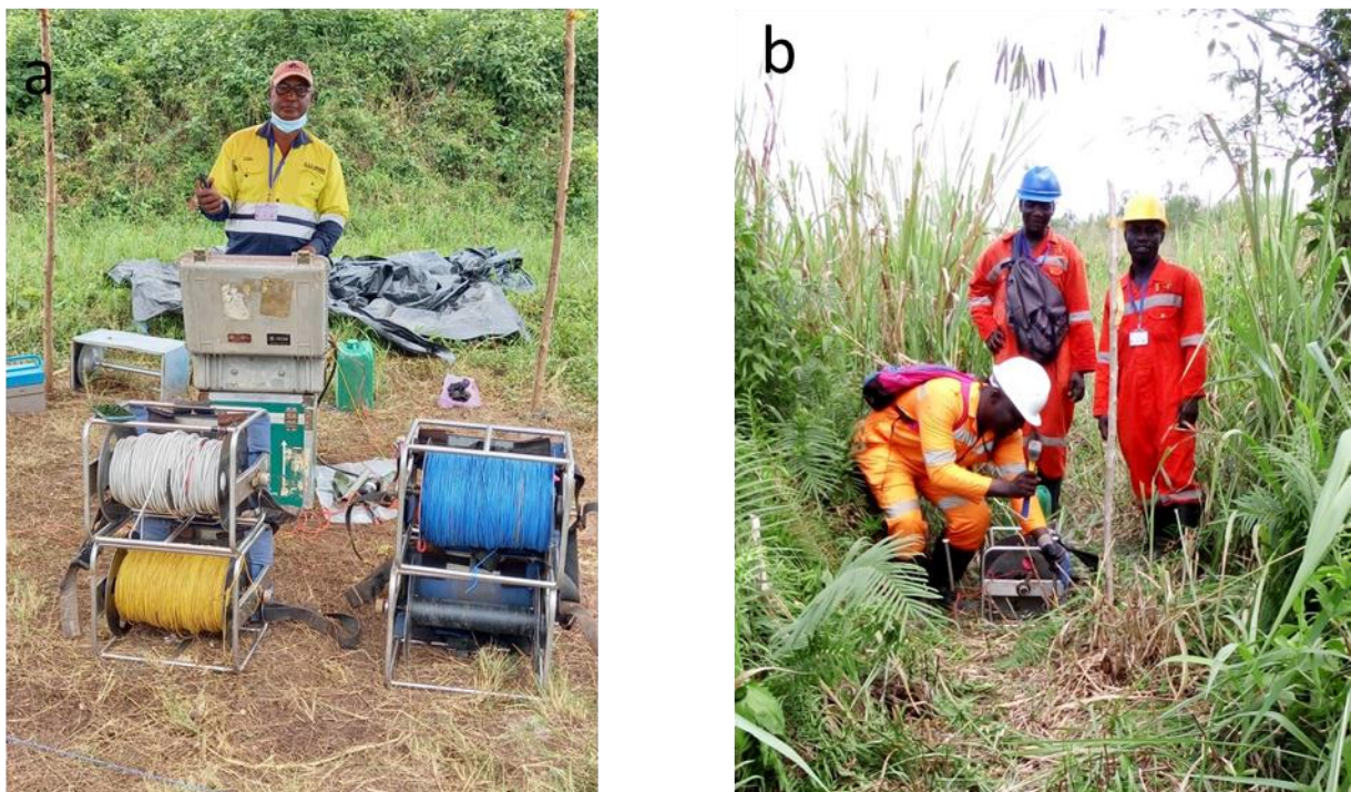
Figure 9-2: (A) Transmitter Operator; (B) IP Survey Current Injection Rods Being Applied
