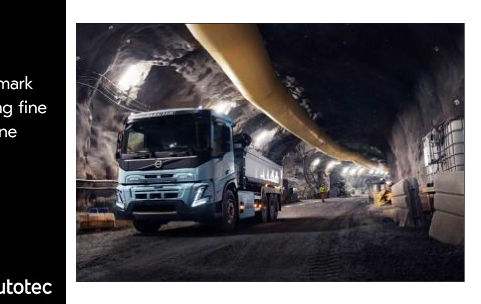
Swedish mining group Boliden is becoming one of the first in the world to start using batteryelectric trucks for heavy underground transport starting 2023. In mining environments, the electric trucks can deliver several big advantages – including no exhaust emissions, a safer workplace, and quieter working conditions.
