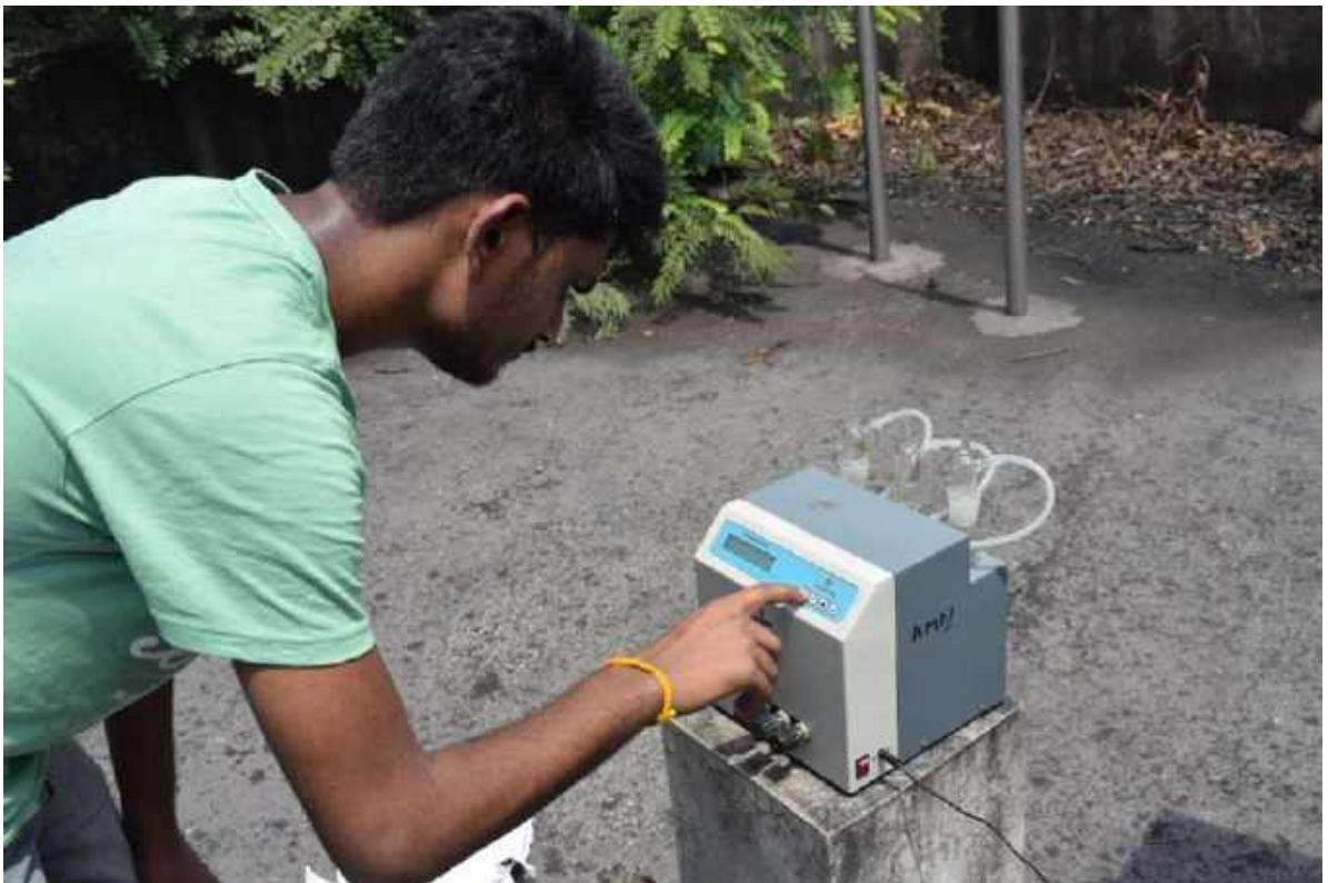
Fig. 4.14: The Uniphos sampler for atmospheric pollutants
