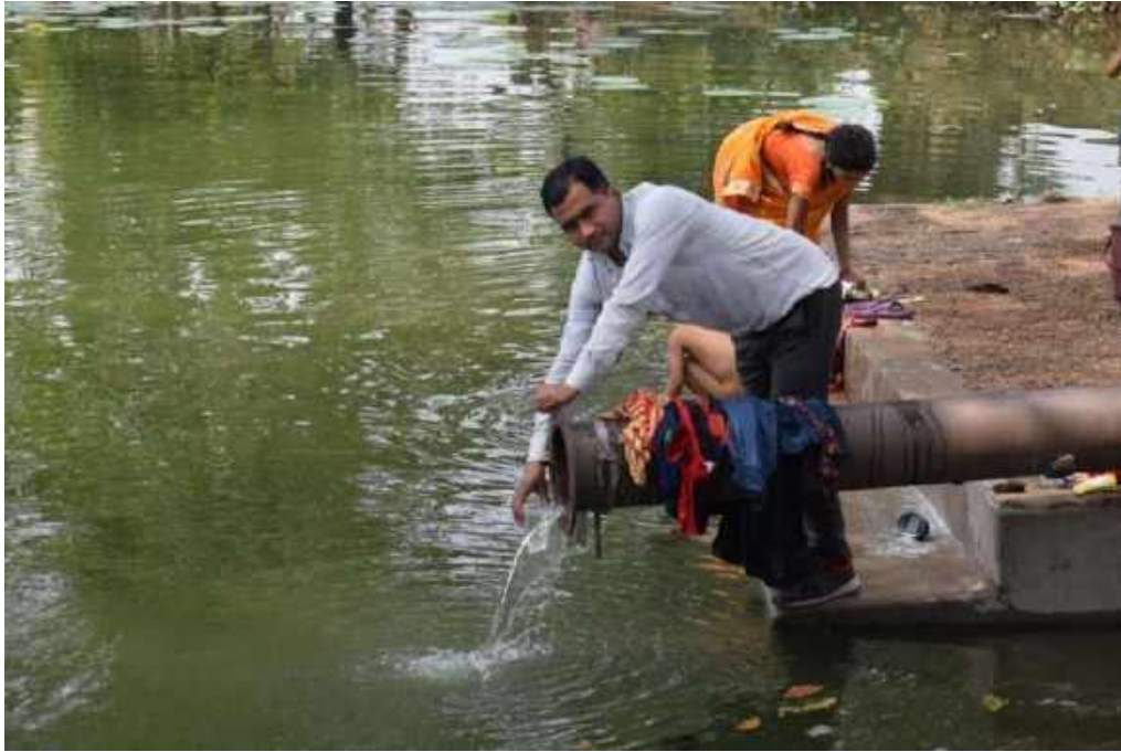
Fig.4.1:- Water sampling from the pond of mine water.
