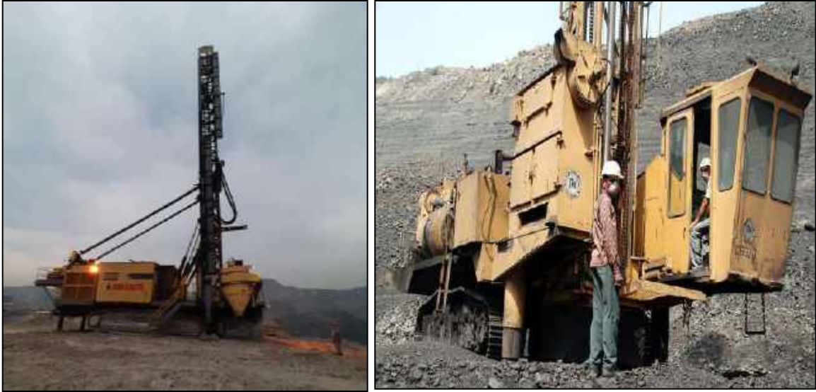
Fig 4: Drill machine with dust extractors
