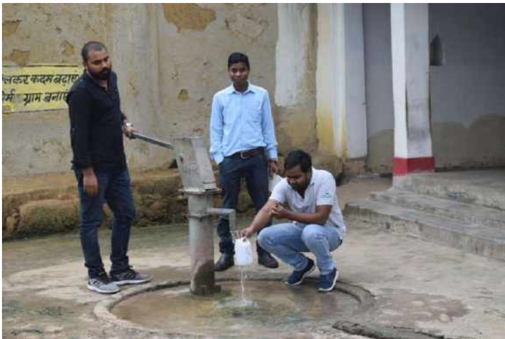
Fig.4.4:- Water sampling from Ground Water (Hand-Pump)
