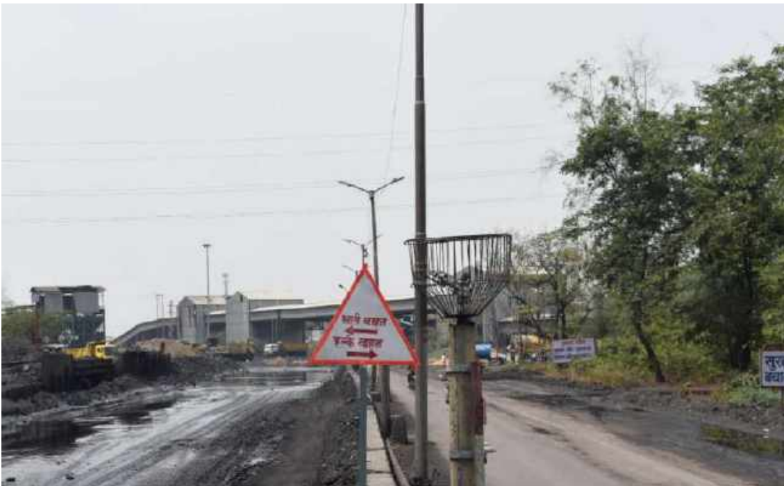
Fig.2.9: Separate roads for transportation of coal & movement of light vehicles
