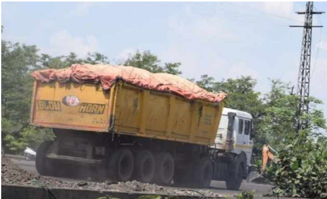
Fig.2.13: Transportation of coal by properly covered truck.
