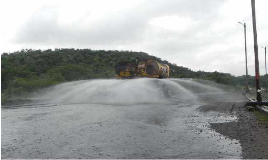
Fig. 2.10: Water spraying through water tank on hall road in mine
