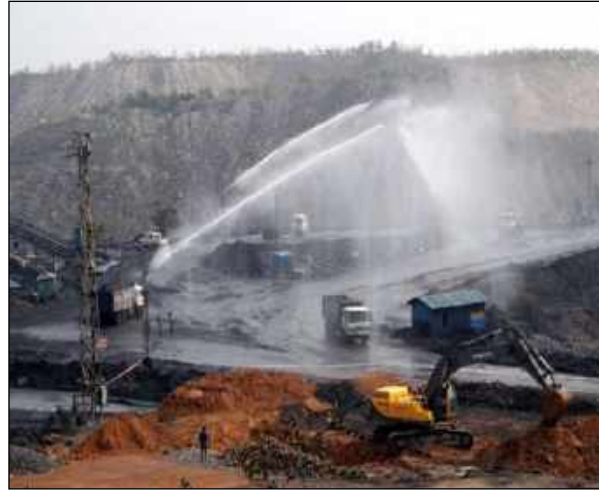
Fig 6: Fixed Sprinklers & Rain Guns for Dust Suppression at Coal Transportation Roads
