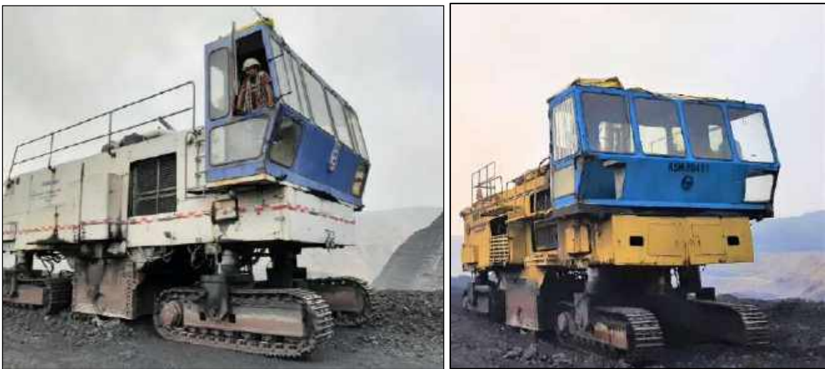
Fig 2: Surface Miner with jet sprinklers for extraction of coal
