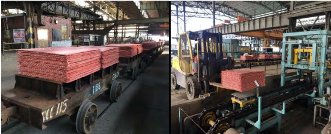
Figure 4. Copper cathode at CSM and existing trolley system.
