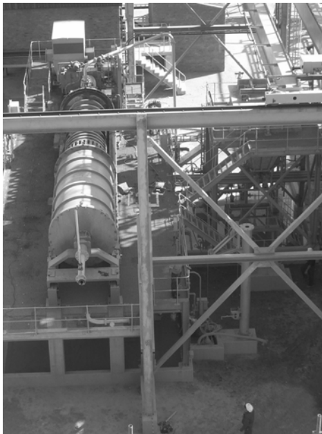
Figure 4: 22 x 11 m footprint of WLTR M10,000 IsaMill grinding circuit
