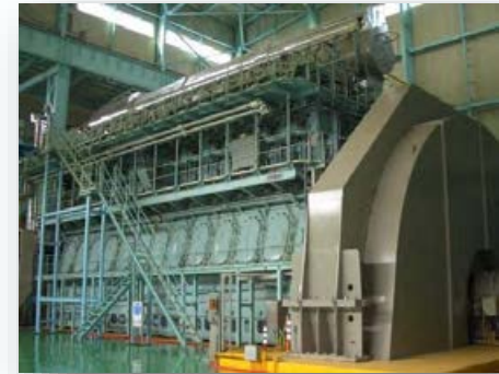
Ultra efficient diesel engine generation
