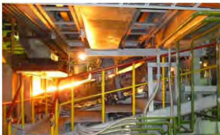
Figure 4 – Tapping matte from the copper ISASMELT at Kazzinc
