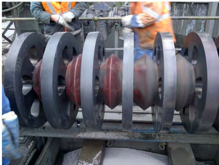
Figure 7 - M1000 IsaMill™ configured with conical spacers
