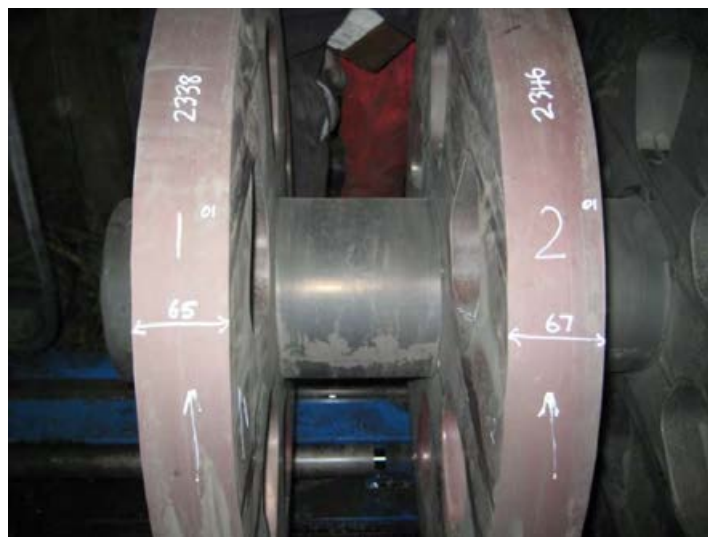
Figure 1 - Conventional Shaft Spacer between two Grinding Discs for an M1000 IsaMill™
