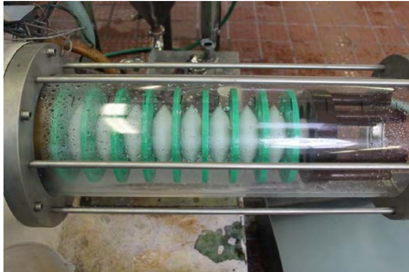
Figure 3 - M20 Clear-Shell IsaMill™, fitted with Conical Spacer Arrangement
