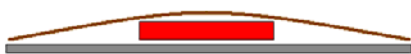
Figure 4 – Thin Wedge, Curved copper due to separation issues on edges due to faulty edge strips
