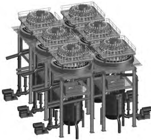
Figure 10: Layout of six B6500/24 model Jameson Cells (Footprint = 22 x 26m; Height = 17m)
