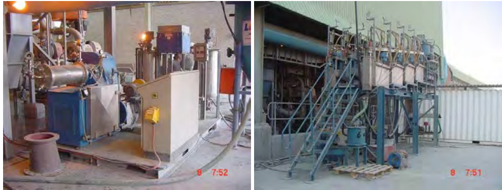
Figure 7: Photographs of the test rig used to evaluate the potential of stirred milling – shown here at Mogalakwena South Concentrator in late 2004
