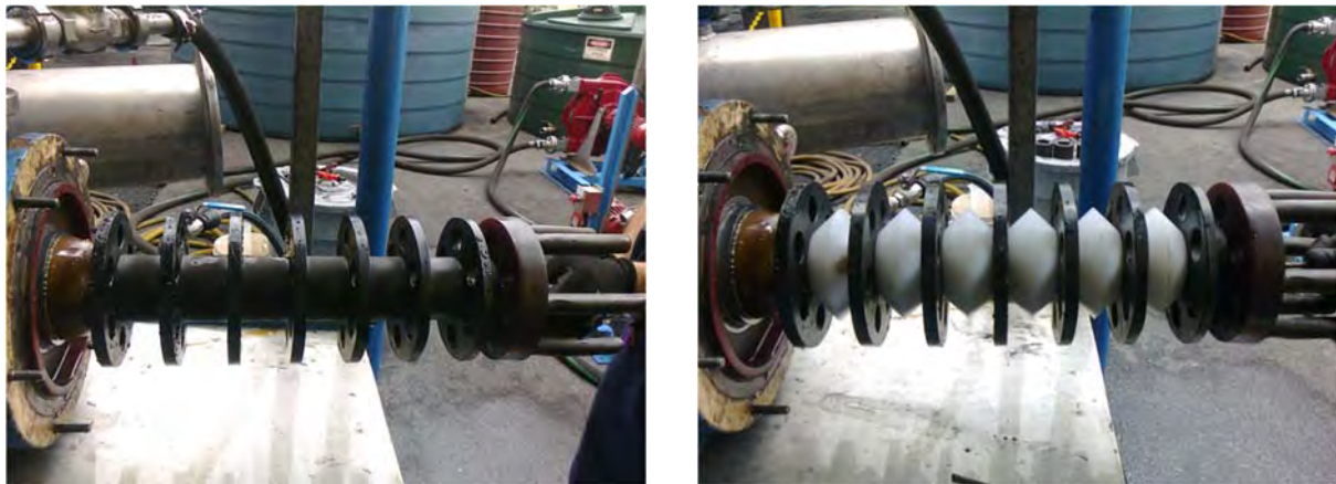
Figure 5 - M20 Pilot Plant IsaMill™ Shaft Configuration with Cylindrical (left) and Conical (right) Spacers
