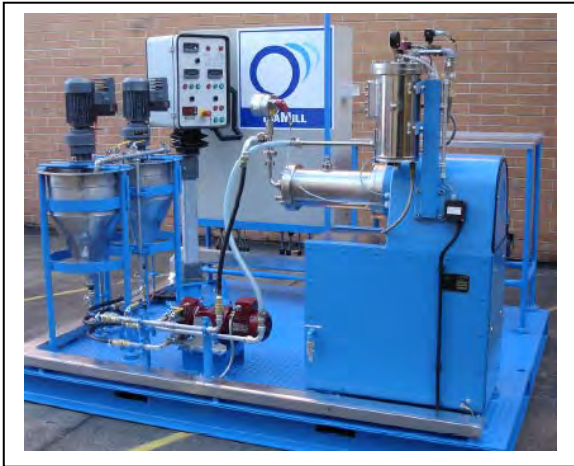
Top: M4 IsaMill™ 4L unit, similar to the unit at CSIRO where testwork was conducted.
