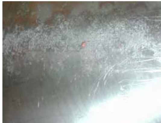
Figure 3: Surface corrosion of the cathode mother plate
