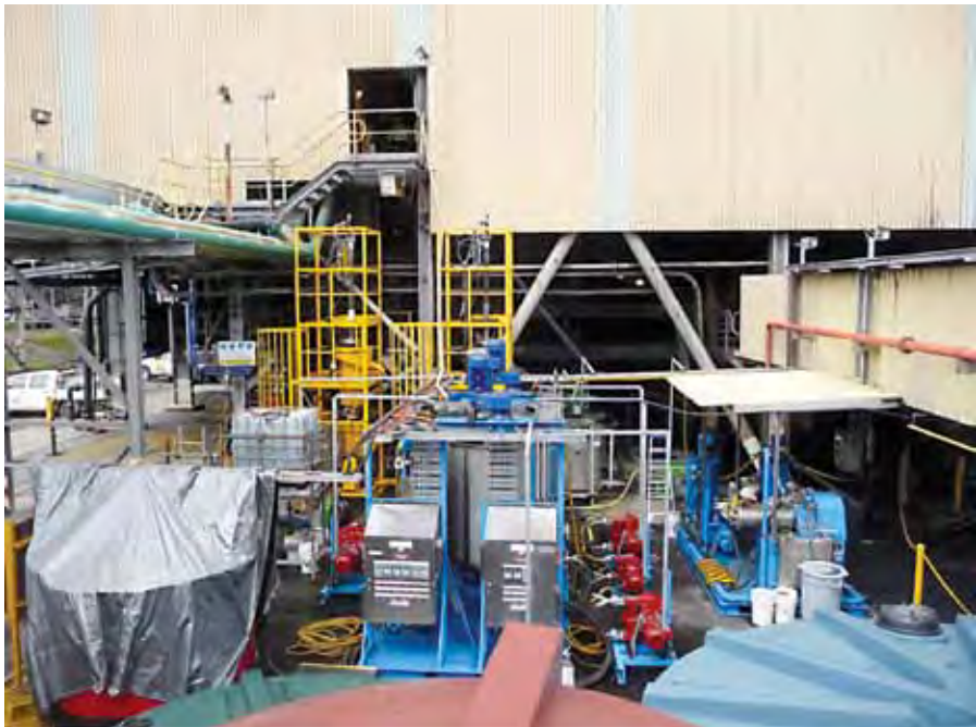
Figure 6 1.0 t/h Coal Tailings Treatment Pilot-plant
