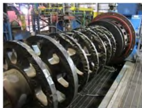
Figure 5 – IsaMill small diameter disc installation from discharge (left picture) and feed (right picture) ends
