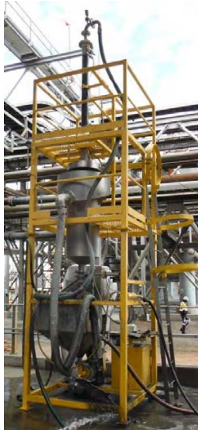
Figure 6 – Jameson Cell L500 pilot plant test rig at Lumwana site
