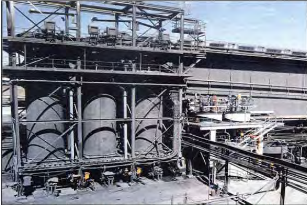
Figure 6 – Jameson Cells compared to columns of the same capacity at Mount Isa
