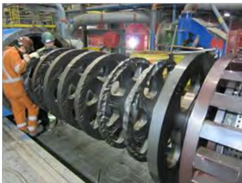
Figure 5 – IsaMill small diameter disc installation from discharge (left picture) and feed (right picture) ends
