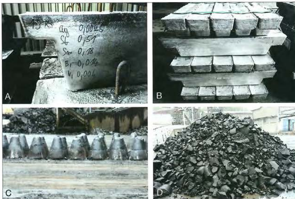
Fig. 5: A – bullion lead; B – refined lead; C – ingots: slag with matte; D – matte [10]
