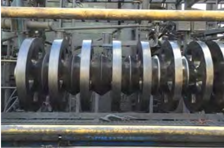
Figure 13 - M1000 IsaMill™ with Conical Spacers after 375 hours of Operation
