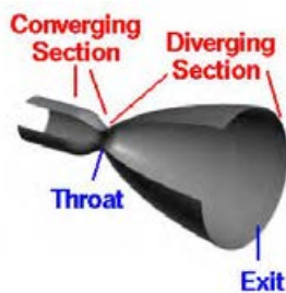
Figure 3 Cross section of a convergent-divergent nozzle (NASA, 2015)
