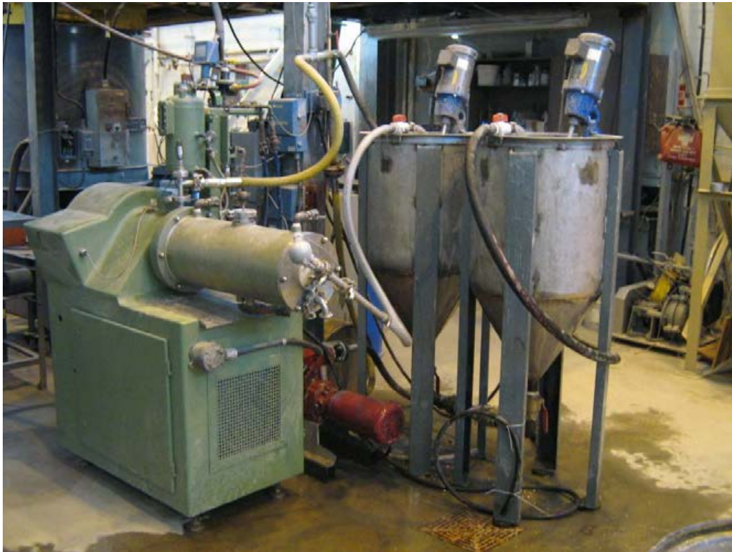
Figure 7 – M20 stirred mill installation at the NBK Institute of Mining
