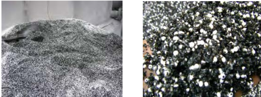
Figure 14: Photographs show severe critical size build up in the IsaMill™ at Mogalakwena South A and B sections; the media is white and the coarse feed particles are generally dark coloured
