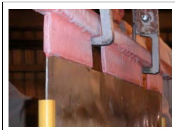
Figure 1: ISA Cathode BR™ in service at Compania Minera Zaldivar
