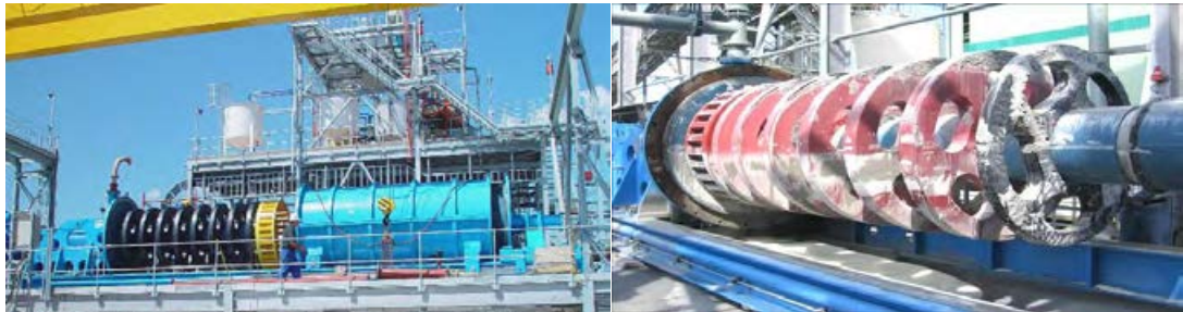
Figure 13: Internals of the IsaMill™, shows the grinding discs and separator with mill shell pulled back on the sliding rails – access position during maintenance
