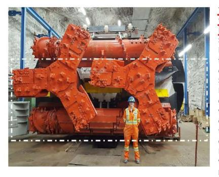
The ultra large borer miner the cable-powered Sandvik MF460 - will be teamed with a Sandvik PO140 EBS. This integrated system is notable for being much larger than other mining machines in the Saskatchewan Potash basin. Four of these systems, developed in close cooperation with Sandvik, will each be capable of about 2.7 Mt for a total potential production capacity of 10.8 Mt/y. The MF460 led system means less workers, so a lower labour cost per tonne, but also a lower
