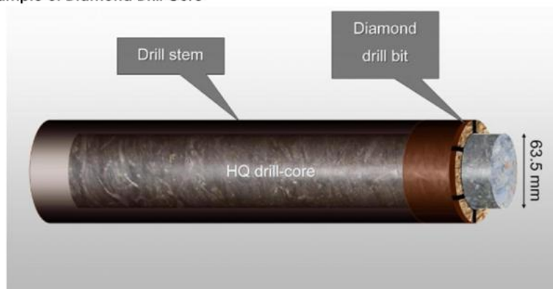
HQ drill-core with drill bit and stem
