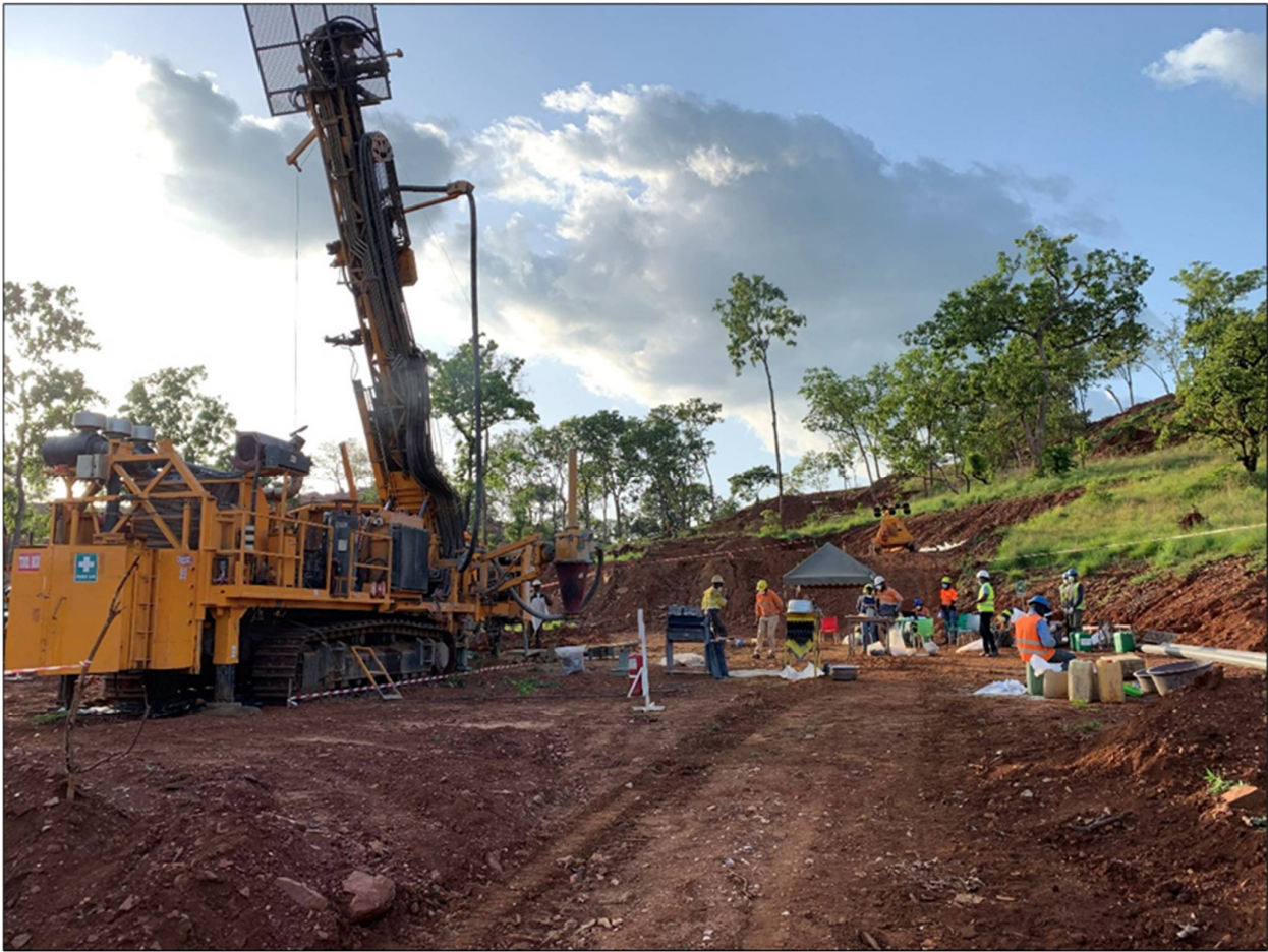
Figure 10-3: RC Drill Rig (Hole ID: LFRC21-1405) and Associated Sampling Setup
