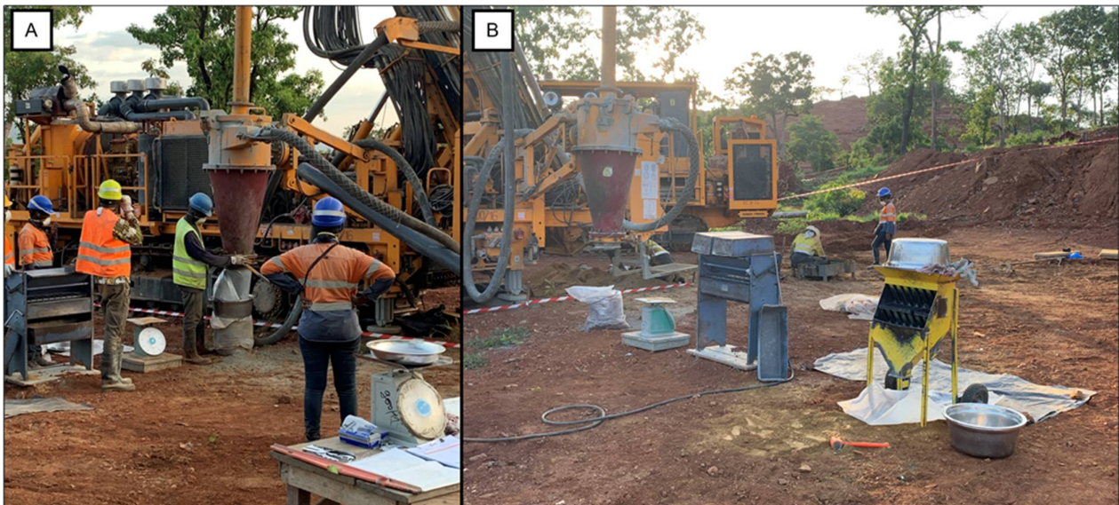
Figure 11-1: Photographs Showing Sampling Procedures at an RC Drill Rig
