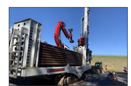
Borterra says RodBot™ robotic drill-rod handling supercharges productivity and boosts safety
