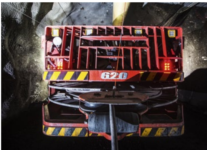
One of Toro LH625iE’s many new features is the re-engineered cable reeling system, designed to increase trailing cable lifetime.
