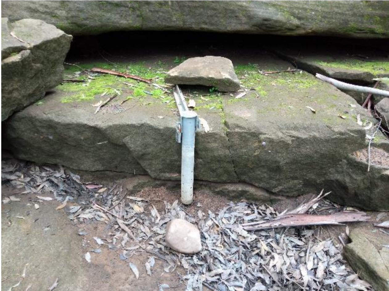
Figure 14: Water Level Monitoring Device at Pool 20 (M20)
