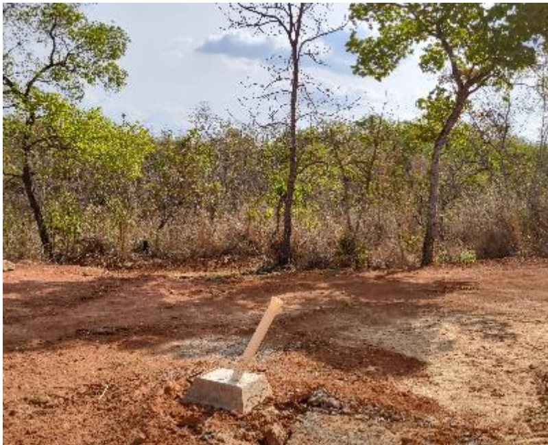
Figure 29 - Data verification: Drill hole collar landmark location
