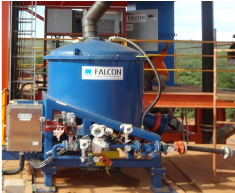
Figure 94 - Falcon centrifugal concentrator overview
