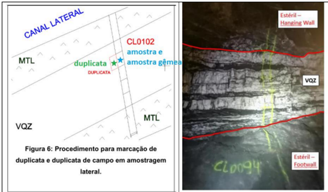
Figure 17 - Procedure of channel sampling in Santo Antônio vein (Xavantina, 2022)
