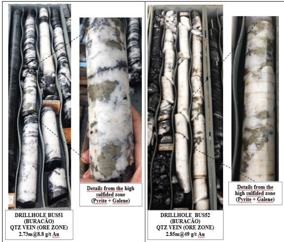
Figure 10 - Quartz vein with high sulfidation (Pyrite and Galena) and high gold grade (Xavantina, 2018)
