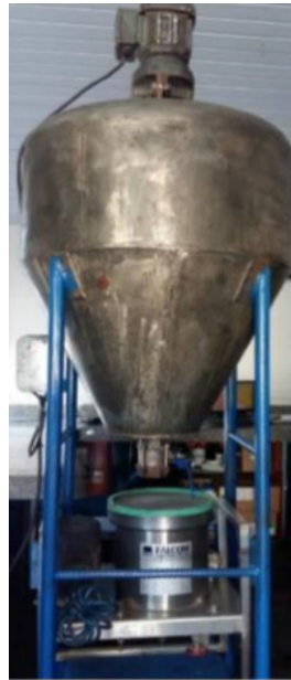
Figure 44 - Falcon Concentrator L40 - Laboratory Size
