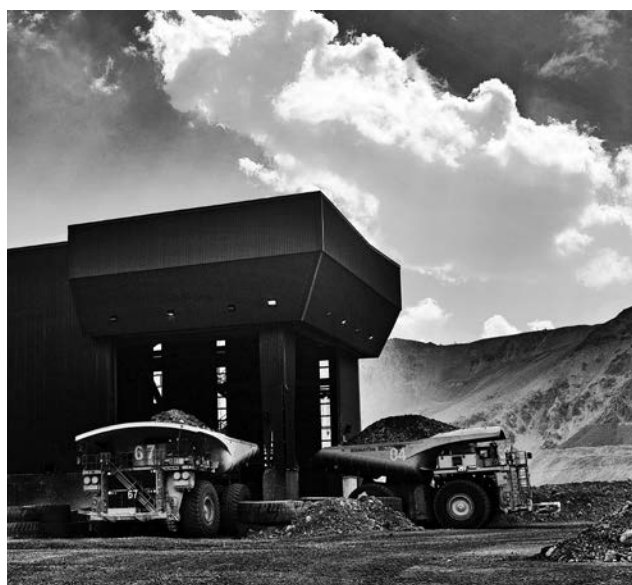
Haul trucks unload ore at the primary crusher in Los Bronces' open pit.
