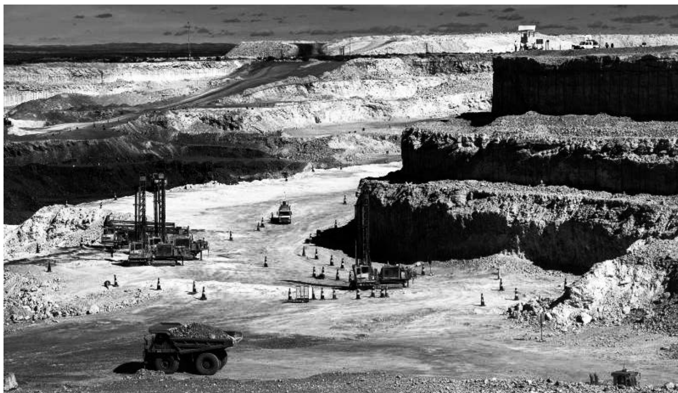
Drilling, loading and hauling activity in Kumba Iron Ore's open pit at Kolomela, South Africa.
