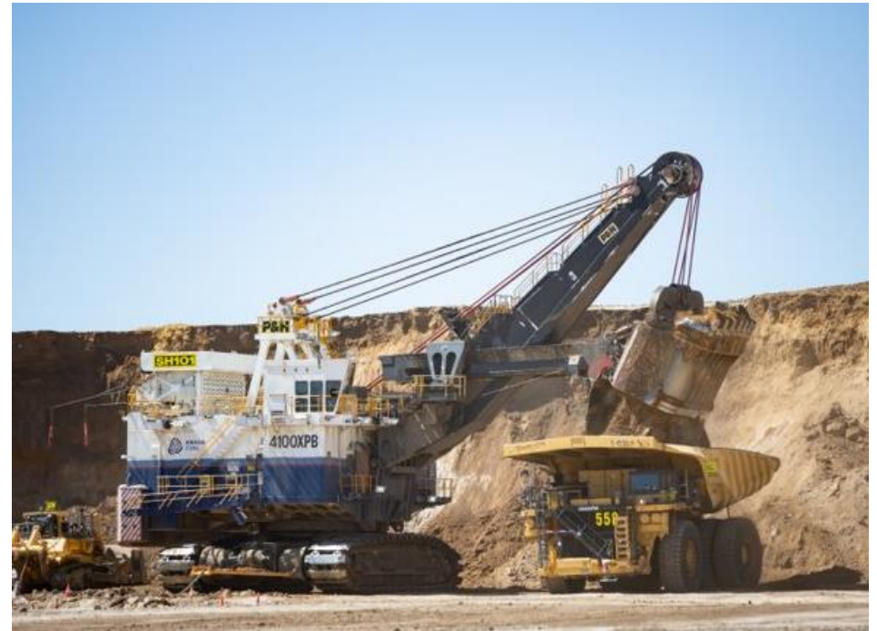
Capcoal's 4100 shovel produced at a 42Mt annualised run rate in 2018 - Anglo American's best performing shovel for the year
