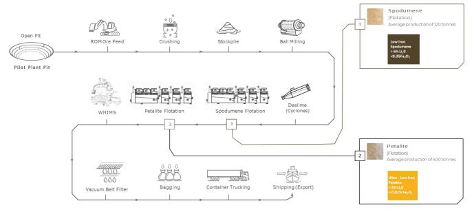
Figure 1 Block Flow Diagram
