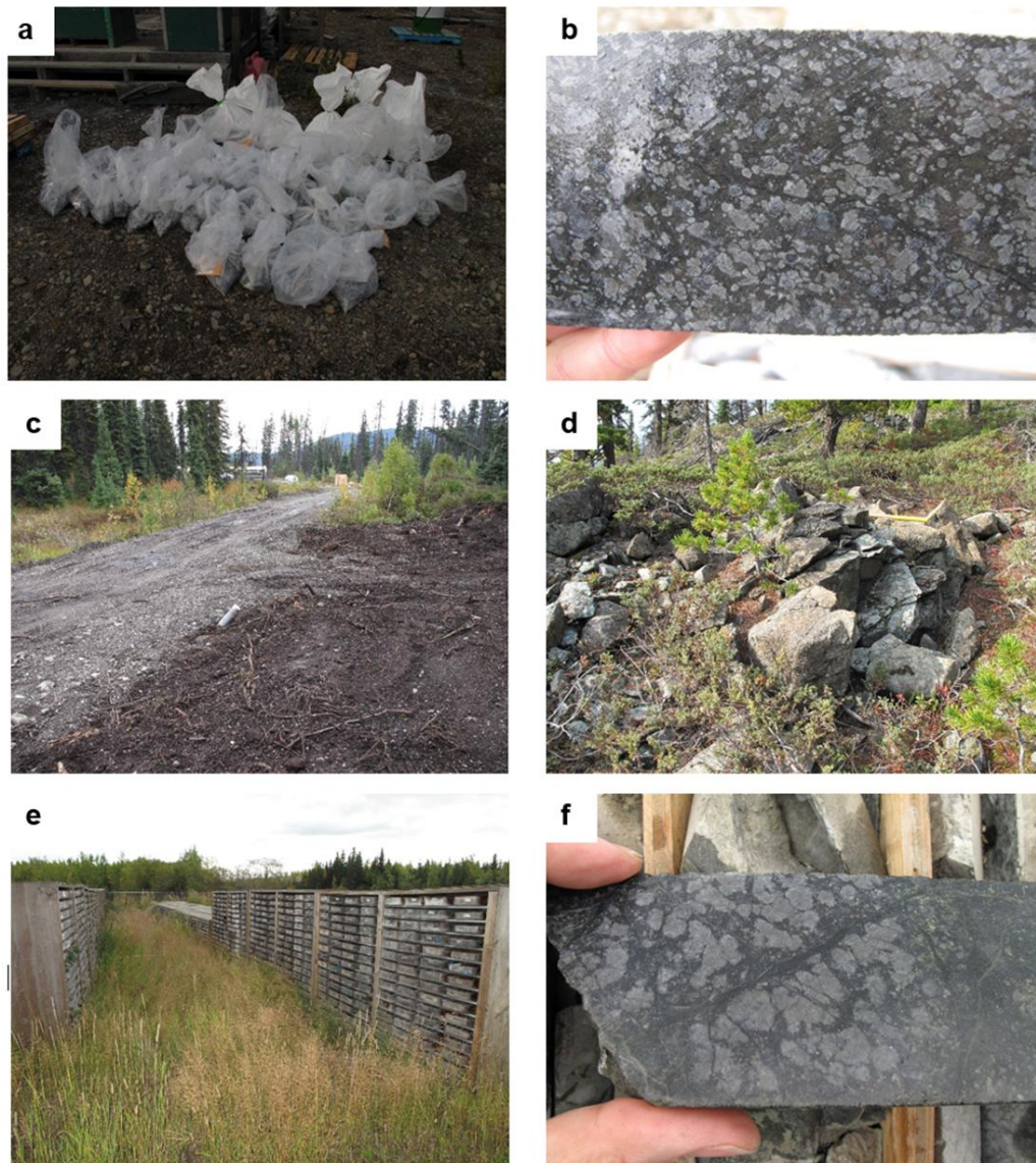
Figure 12-1: Photos from Voordouw’s 2017 site visit that show (a) poly-ethylene bags with samples from 17BAP070, (b) awaruite mineralization in serpentinized peridotite, 17BAP067 at approximately 125 m depth, (c) reclaimed drill pad and casing for 17BAP068, with camp in the background, (d) outcrop of peridotite at northwest end of Baptiste Deposit, (e) part of the historical core storage yard in Fort St. James, and (f) serpentinized peridotite with high-grade awaruite mineralization at 85 m depth. Source: photographs by Ron Voordouw (2017).
