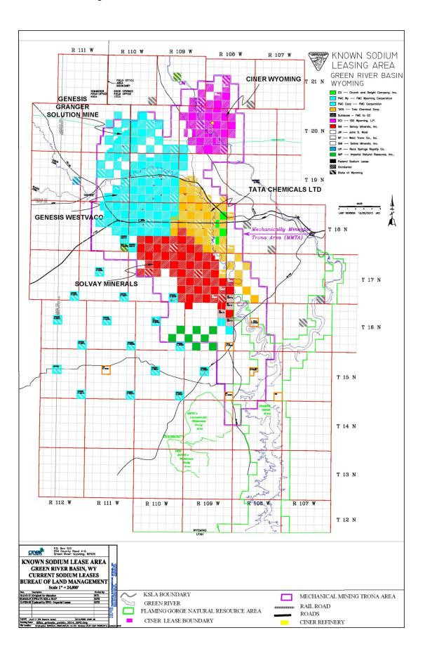
The Green River Basin geological formation holds the largest, and one of the highest purity, known deposits of trona ore in the world. Our reserves contain trona deposits having a purity between 80% to 89% by weight, which means that insoluble impurities and water make up approximately 11% to 20% of our trona.
