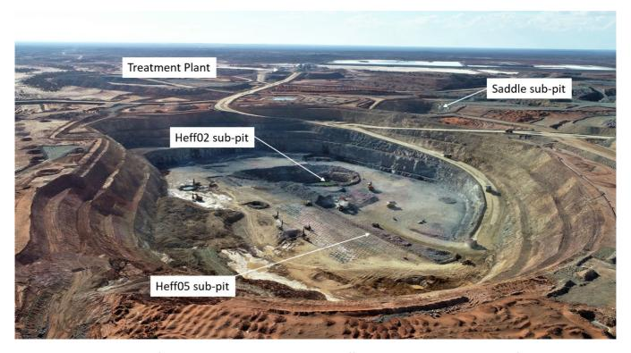
**Figure 2:** Photograph of Current Mining Activities at the Heffernans Pit Showing Location of the Completed Saddle and Heff02 Sub-pits; and the Heff05 Sub-pit
